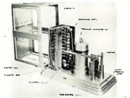
Fig. 12. Pressure unit for an automatic weather station.
