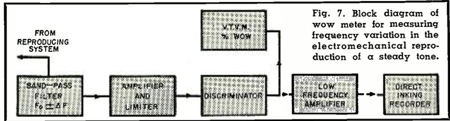
Fig. 7. Block diagram of wow meter for measuring frequency variation in the electromechanical reproduction of a steady tone.
