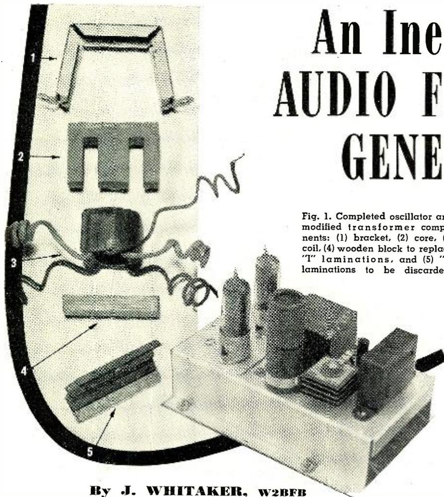
Fig. 1. Completed oscillator and modified transformer components: (1) bracket, (2) core, (3) coil, (4) wooden block to replace "I" laminations, and (5) "I" laminations to be discarded.
