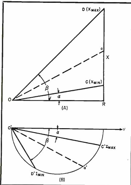
Fig. 9. (A) Impedance diagram and (B) admittance or current diagram for simple magnetic amplifier.
