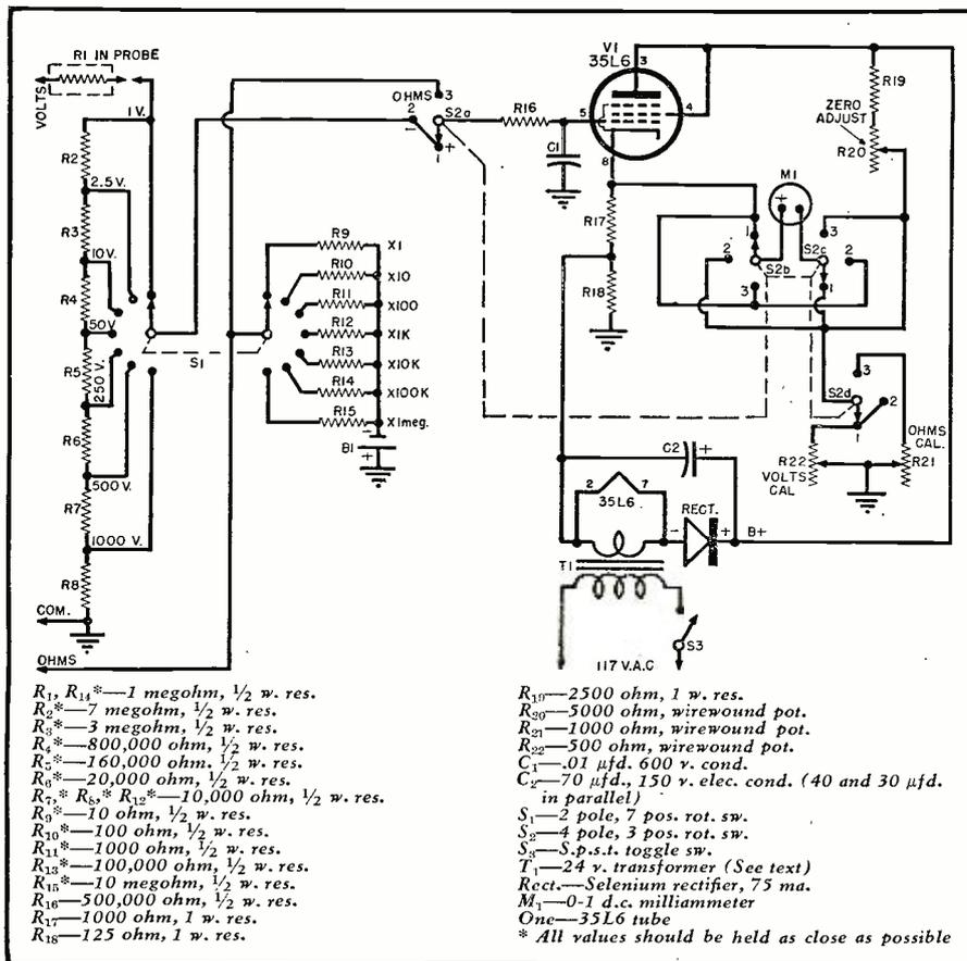
The 35L6 tube is used as a cathode follower in this v.t.v.m.-ohmmeter. The v.t.v.m. circuit as it is shown in diagram can be used only for d.c. voltage measurements.
