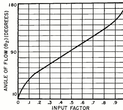
Fig. 12. Angle of flow on current waveform vs. relative input factor. Maximum flow is 180 degrees.
