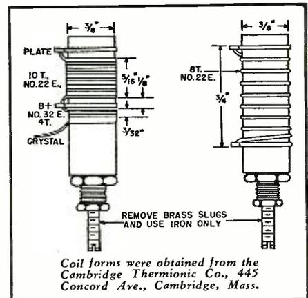
Mechanical details of coil assemblies. Coil  $L_1$  is on left and  $L_2$  is on right.
