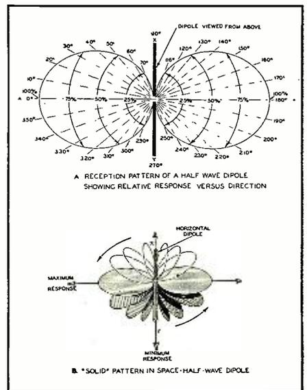
Fig. 8. The reception pattern in space of the basic half-wave dipole antenna.
