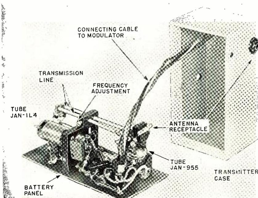
Fig. 8. Partly disassembled view of 1700 mc. radiosonde transmitter.
