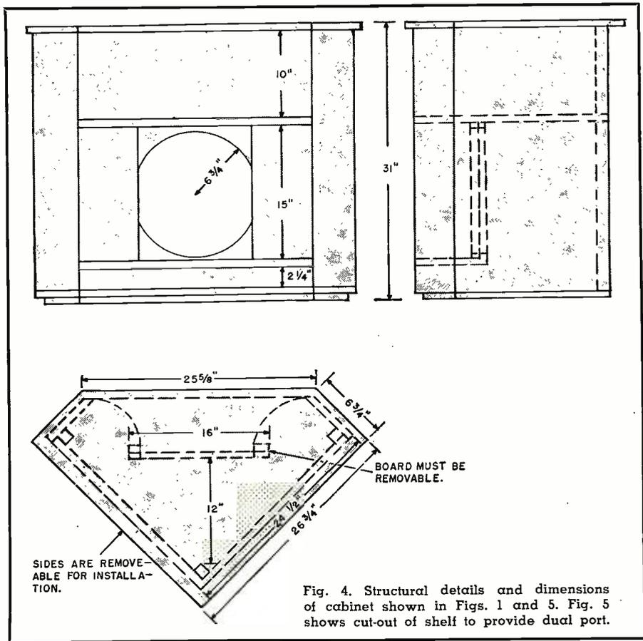
Fig. 4. Structural details and dimensions of cabinet shown in Figs. 1 and 5. Fig. 5 shows cut-out of shelf to provide dual port.
