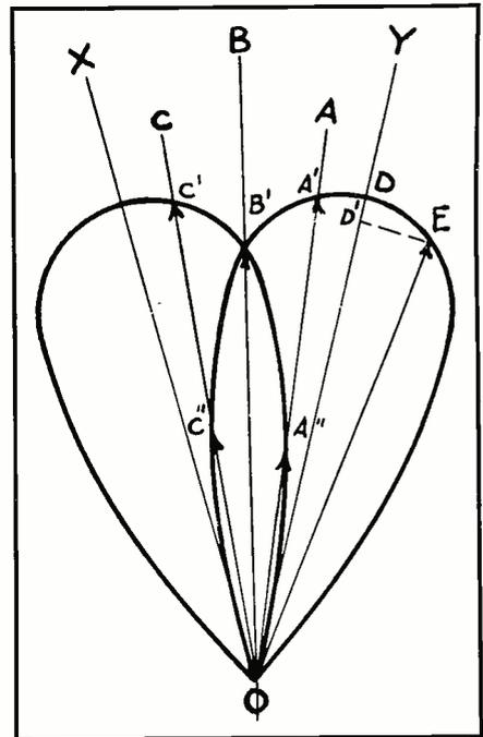
Fig. 7. Split pattern, or lobe switching, tracking.
