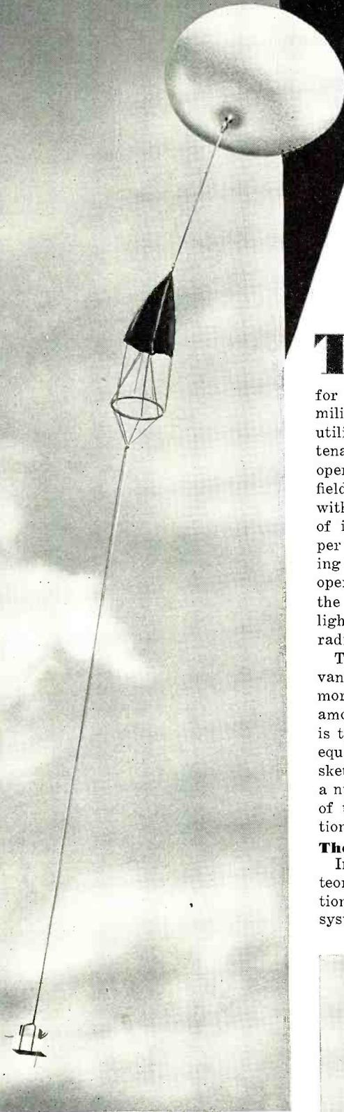
Fig. 1. The radiosonde is carried aloft by a balloon. When the balloon bursts, the equipment is lowered to the ground by means of a parachute.
