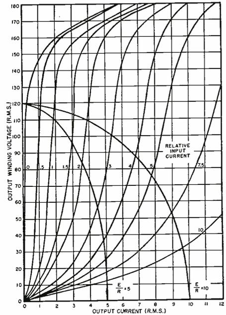
Fig. 6. Output winding reactance vs. input current as based on the slopes of the curves at the origin of Fig. 4.
