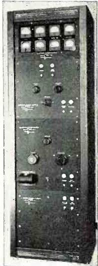
The first three units, beam supply, reflector supply, and control electrode supply, delivering d.c. power are well regulated. The fourth unit, filament supply delivering a.c. power, is not regulated.
