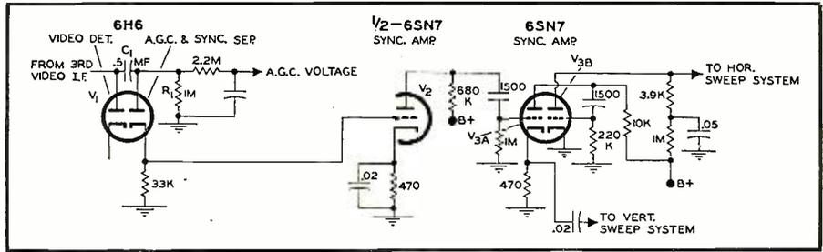
Fig. 6. Diagram showing a combination sync separator and a.g.c. rectifier.
