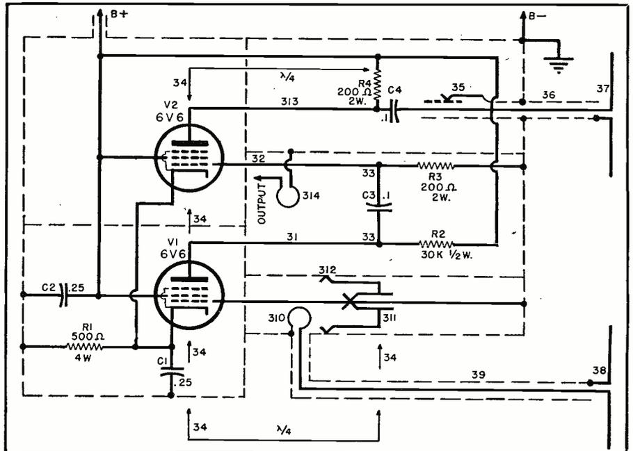
V<sub>1</sub>, the coupling circuit (31-32), and plate output circuit (313) are separated by a complete and careful system of shields in order to prevent coupling other than the space coupling between the dipoles (37 and 38). Chassis currents and the common power supply always provide a small coupling which in any case can sustain the oscillation. The tubes may be energized at the approximate voltages recommended by the tube manufacturer for such type.
