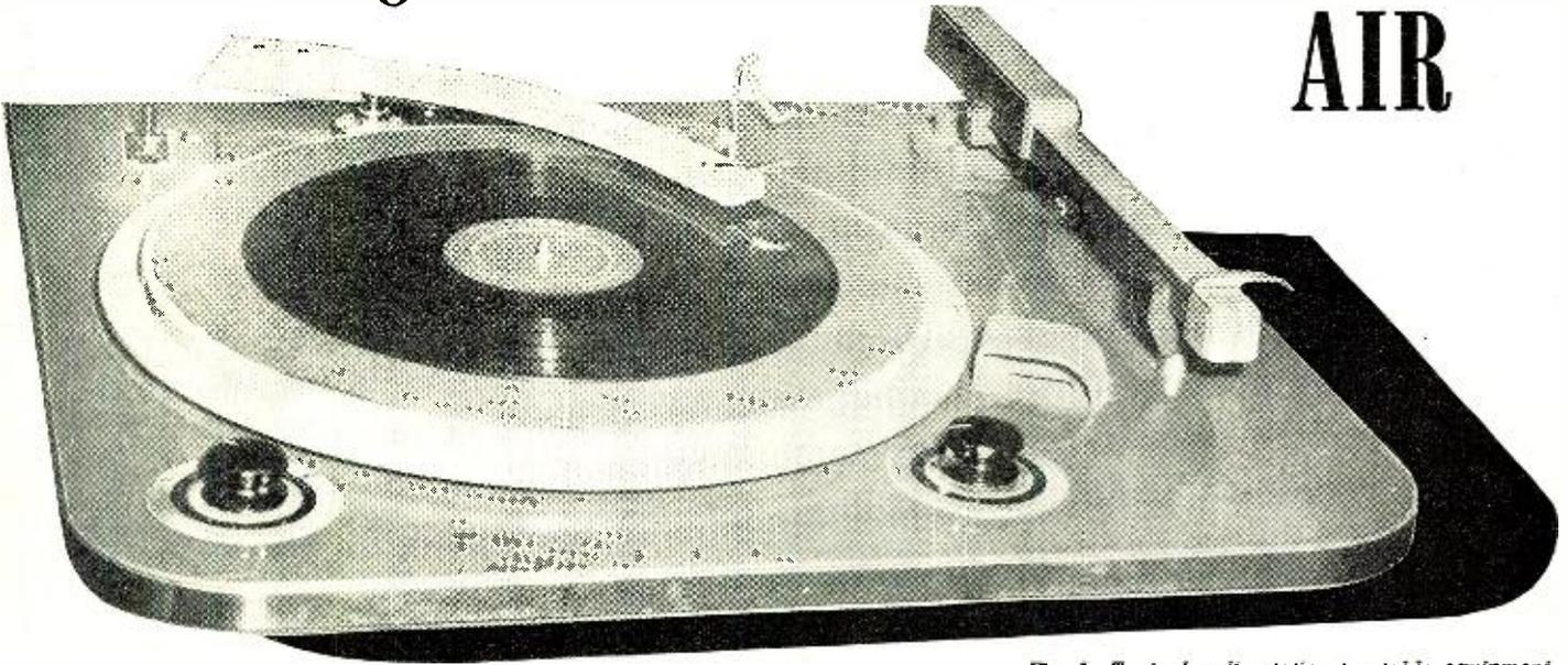
Fig. 1. Typical radio station turntable equipment, adapted for microgrooves. Note conventional pickup arm at right and changeover switch, left rear.
