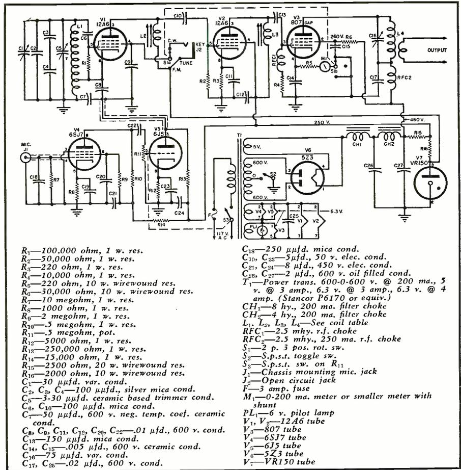
Complete diagram of transmitter, including its self-contained power supply.
