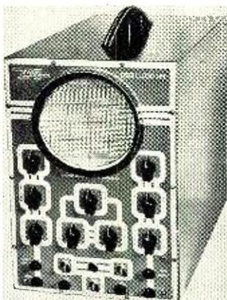
It provides for external synchronization, test voltage, and intensity modulation.
