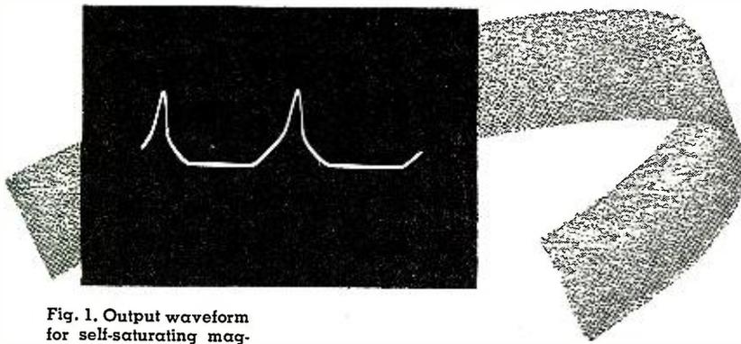
Fig. 1. Output waveform for self-saturating magnetic amplifier with input factor of about 0.2.
