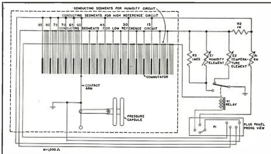
Fig. 4. Schematic diagram of the radiosonde modulator.
