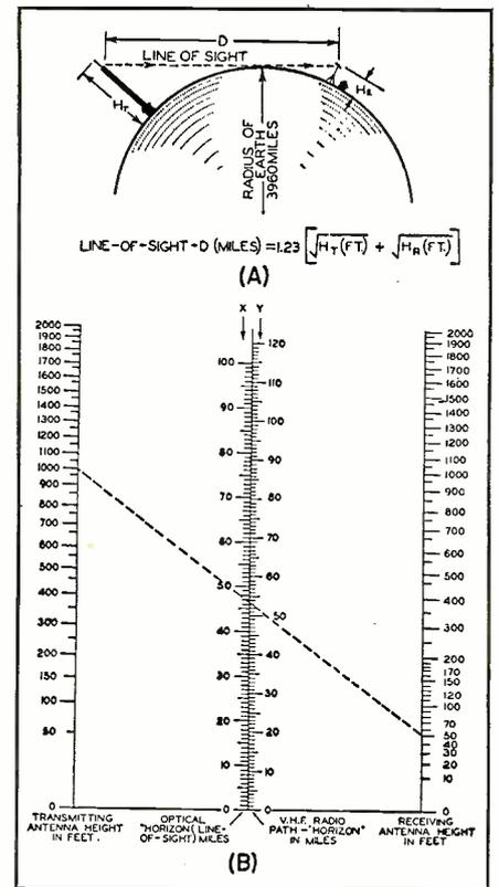
Fig. 3. V.h.f. path length as a function of height of transmitting and receiving antennas. (A) Line-of-sight. (B) Theoretical maximum line-of-sight path chart. The v.h.f. radio path is equal to the optical horizon distance times 1.156. Example: Transmitting antenna, 1000 feet high; receiving antenna, 50 feet high; optical horizon, 46.5 miles—the v.h.f. wave path is then equal to 53.5 miles.
