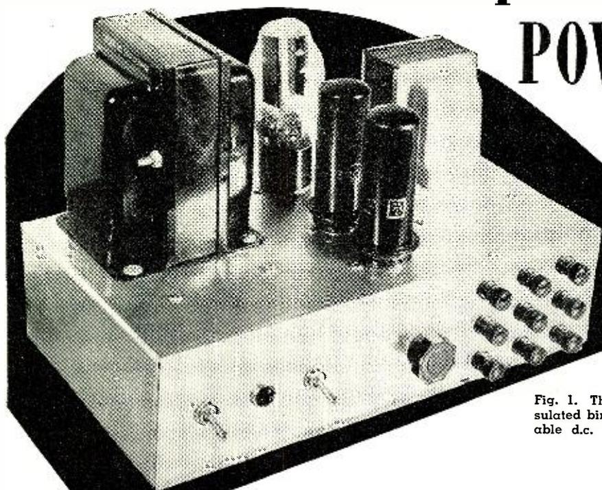
Fig. 1. The d.c. voltage control knob is in the center. Insulated binding posts on the right allow easy access to variable d.c. voltage and to a selection of low a.c. voltages.
