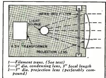
Fig. 4. Light source assembly. Unit contains the light, infrared filter, projection lens, and a filament transformer.
