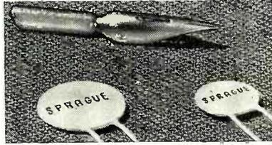
sized ceramic plate of extremely high dielectric constant with silvered electrodes fired on both disc faces, the condensers are coated with a tough, moisture-resistant insulating resin.
