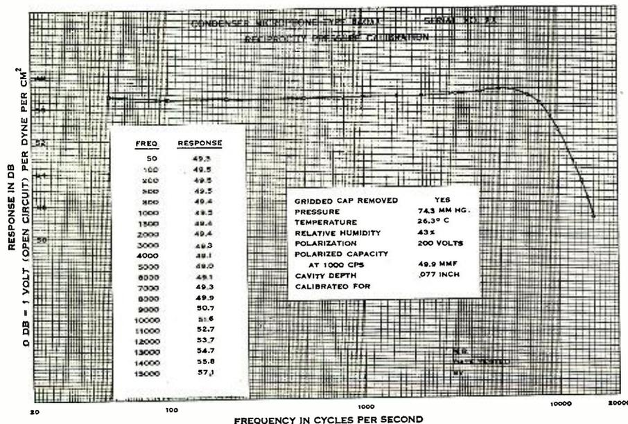
picked up by both the microphone under test and by the standard microphone. Comparison of the output of the two microphones then immediately gives the characteristics of the unit under test.
