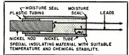
Fig. 3. Probe construction.
