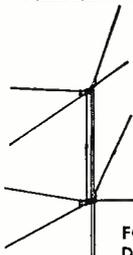
Bi-Directional Stacked Conical "V" Beam
