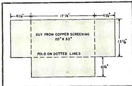
Fig. 4. Details for cutting wire screening.
