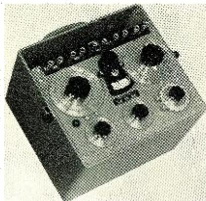
capacitance, and inductance over the following ranges: Resistance, 1 milliohm to 1 megohm; capacitance, 1  $\mu$ fd. to 100  $\mu$ fd.; inductance, 1  $\mu$ hy. to 100
