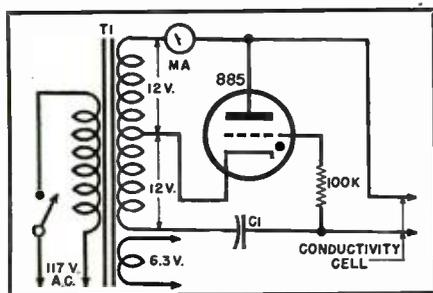
Fig. 5. Phase-sensitive conductivity bridge.  $C_1$  is determined by the probe and solution characteristics. It may range from .001 to 10 mfd.
