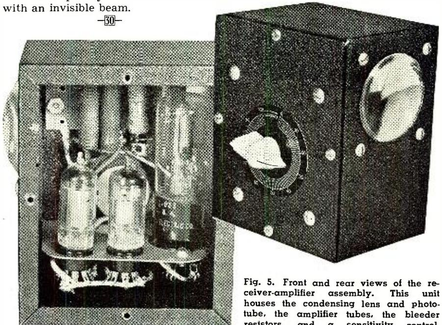
Fig. 5. Front and rear views of the receiver-amplifier assembly. This unit houses the condensing lens and phototube, the amplifier tubes, the bleeder resistors, and a sensitivity control.
