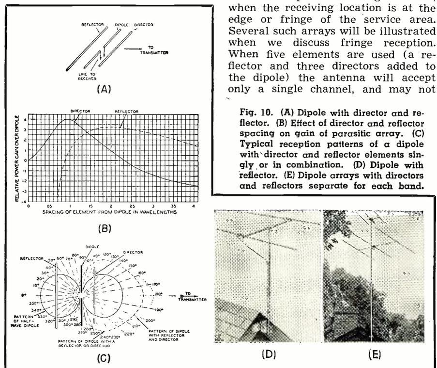
Fig. 10. (A) Dipole with director and reflector. (B) Effect of director and reflector spacing on gain of parasitic array. (C) Typical reception patterns of a dipole with director and reflector elements singly or in combination. (D) Dipole with reflector. (E) Dipole arrays with directors and reflectors separate for each band.
