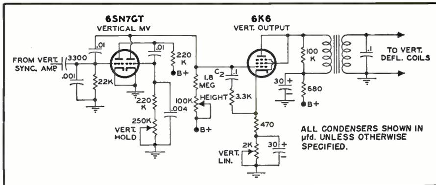
Fig. 8. A vertical deflection system feeding a set of deflection coils.
