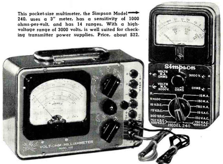
↑ The four-inch meter dominates the case of the Hickok Model 435 volt-ohm-milliammeter, with 35 ranges, a sensitivity of 20,000 ohms-per-volt, and d.c. and a.c. power supplies. Price of unit is about \$38.
