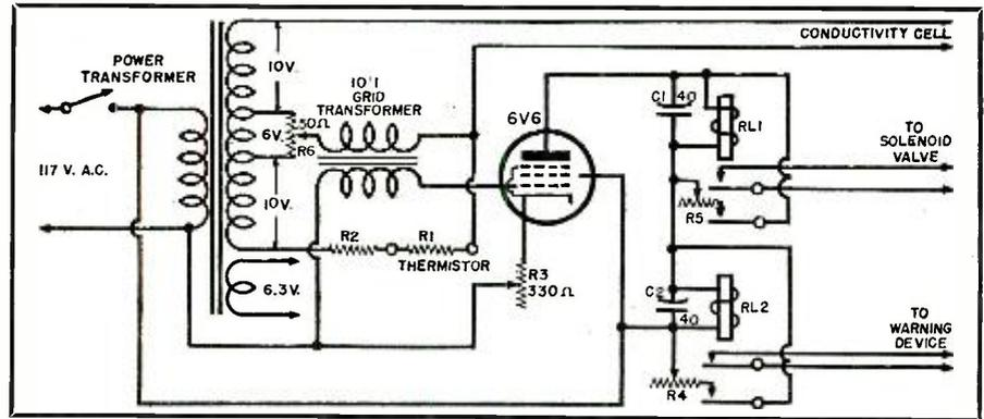
Fig. 2. Complete circuit diagram of the conductivity bridge.
