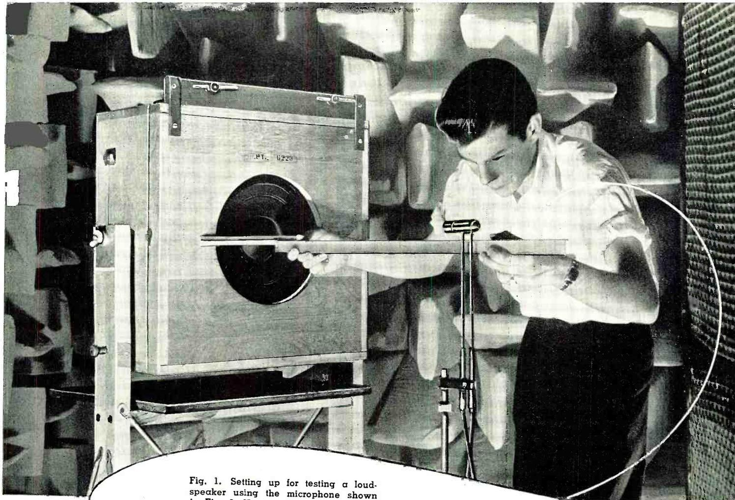
Fig. 1. Setting up for testing a loudspeaker using the microphone shown in Fig. 8. Note accurate placement of microphone with respect to loudspeaker.
