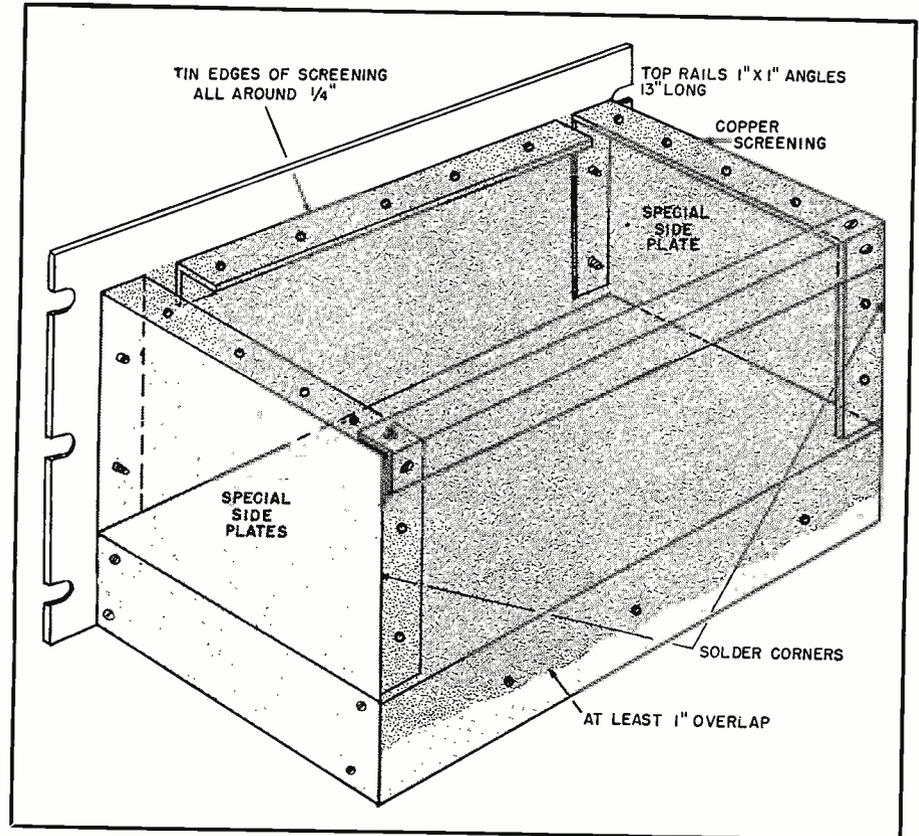
Fig. 3. If chassis supporting brackets are not used special side plates made of aluminum can be used. Copper screening would then be necessary only for top and back.
