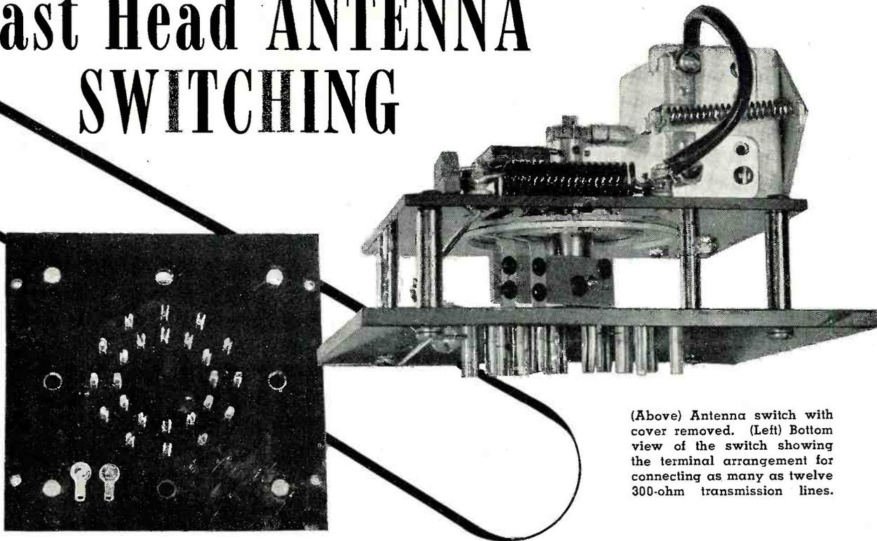
(Above) Antenna switch with cover removed. (Left) Bottom view of the switch showing the terminal arrangement for connecting as many as twelve 300-ohm transmission lines.
