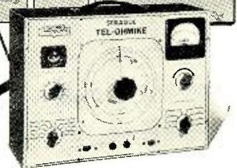
Sprague Tel-Ohmike analyzer for fast, easy testing of all essential capacitor and resistor characteristics.
