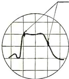
**Two Built-in Markers Can Be Used Simultaneously Giving Facilities for Faster Identification of Bandpass of Curves Without Constant Tuning of Marker**
