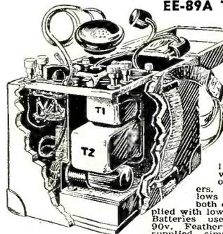
Here's a REAL BUY. Improves transmission and extends talking range of EE-8 and RM29-A telephones. Only 2 wire lines used. Simplex telegraph and 20 cycle ringing possible over 111 c/s equipped with one or more of these repeaters. Hybrid coil allows transmission in both directions. Supplied with low-drain 95 tube. Batteries used: 1 1/2 v. and 90v. Featherweight phone supplier, simple to set up. BRAND NEW. Complete with instruction manual. ONLY \$9.95 ea. Limited quantity.
