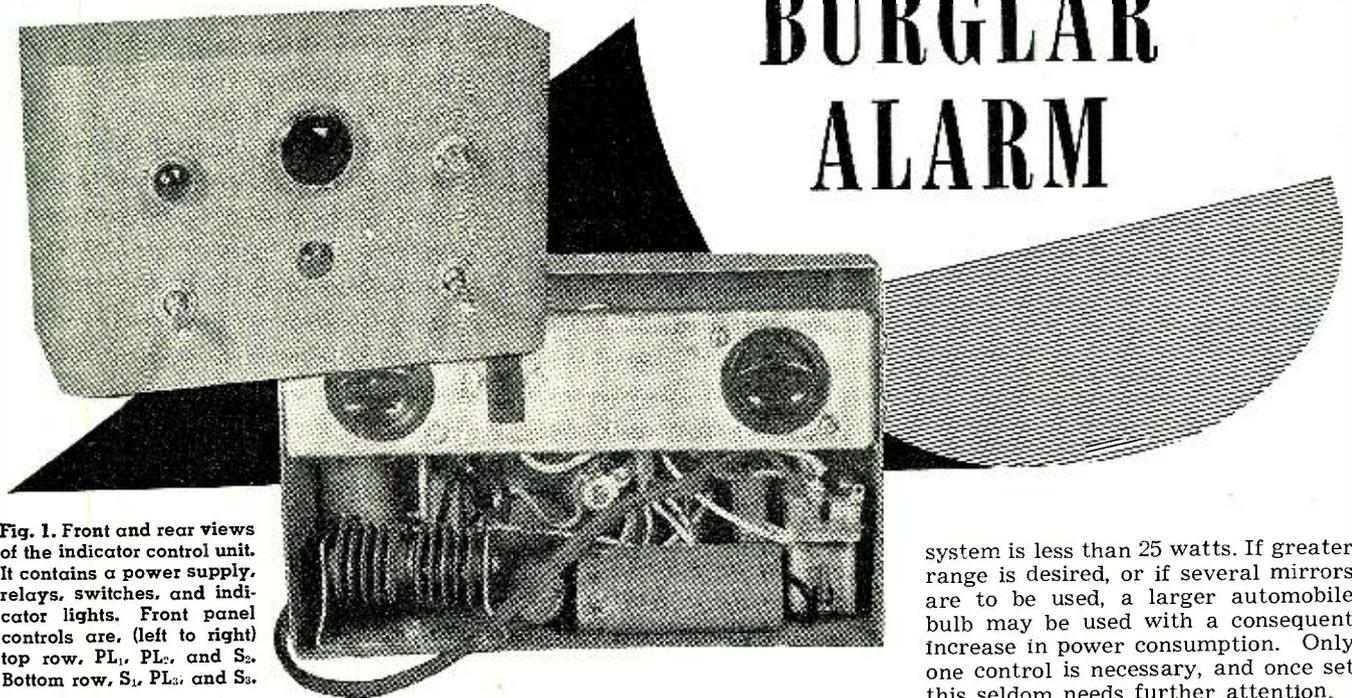
Fig. 1. Front and rear views of the indicator control unit. It contains a power supply, relays, switches, and indicator lights. Front panel controls are, (left to right) top row, PL<sub>1</sub>, PL<sub>2</sub>, and S<sub>2</sub>. Bottom row, S<sub>1</sub>, PL<sub>3</sub>, and S<sub>3</sub>.
