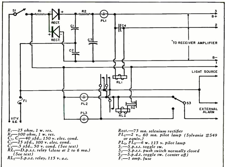
Fig. 3. Wiring diagram of the indicator-control assembly.
