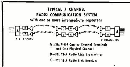
Fig. 7. Typical 7-channel point-to-point communications system utilizing FTL-13-A radio link and six FTR 9-H-1 carrier channels.
