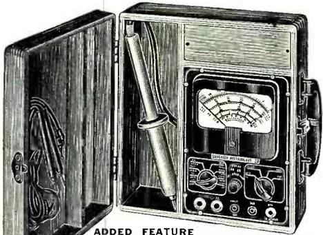
9 D. C. VOLTAGE RANGES: (At 20,000 ohms per Volt) 0-2.5 / 10/50 / 100 / 250 / 500 / 1,000 / 5,000/50,000 Volts
