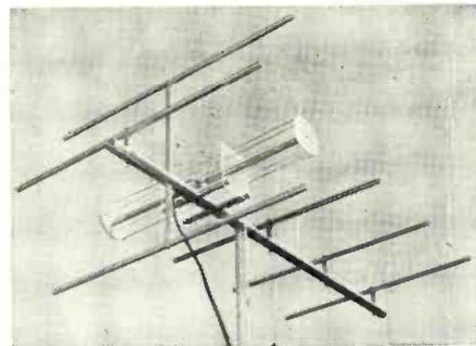
folded cage signal trap to the surge impedance of standard 300-ohm transmission line. Being cut to channel and correctly spaced, it is assured of maximum efficiency for highest gain.
