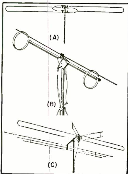
Fig. 15. Three different types of dual-element, wide-band television antennas.
