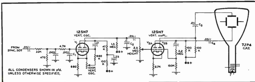
Fig. 2. A widely-used vertical sweep system.
