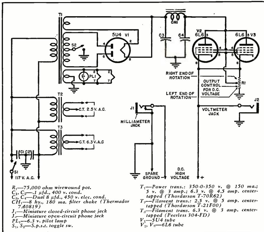
Fig. 2. Complete wiring diagram of the experimenter's low-cost power supply.
