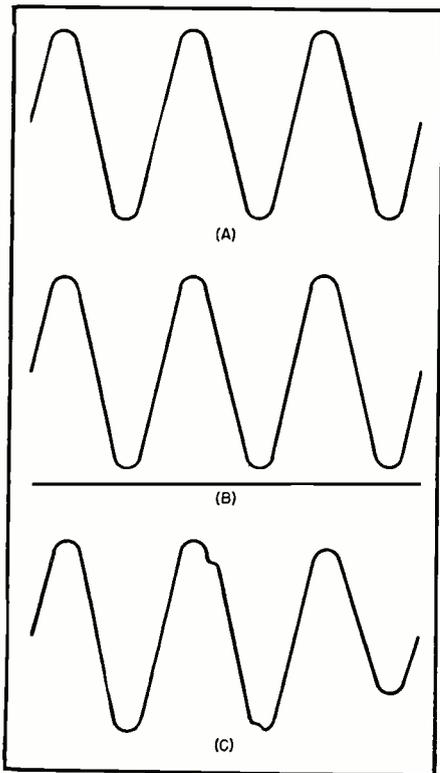
Fig. 2. Patterns observed when line is incorrectly terminated. (A) Phasing adjustment on sweep generator correctly set. (B) Sweep generator blanked during return sweep. (C) Pattern resulting when there is a fault on the line.
