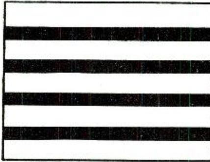
Fig. 2. Number of dark horizontal bars caused by heavy oscillations in the camera chain. In this case the trouble was due to a poor connection in a heater transformer. Resoldering the defective connection corrected the trouble.
