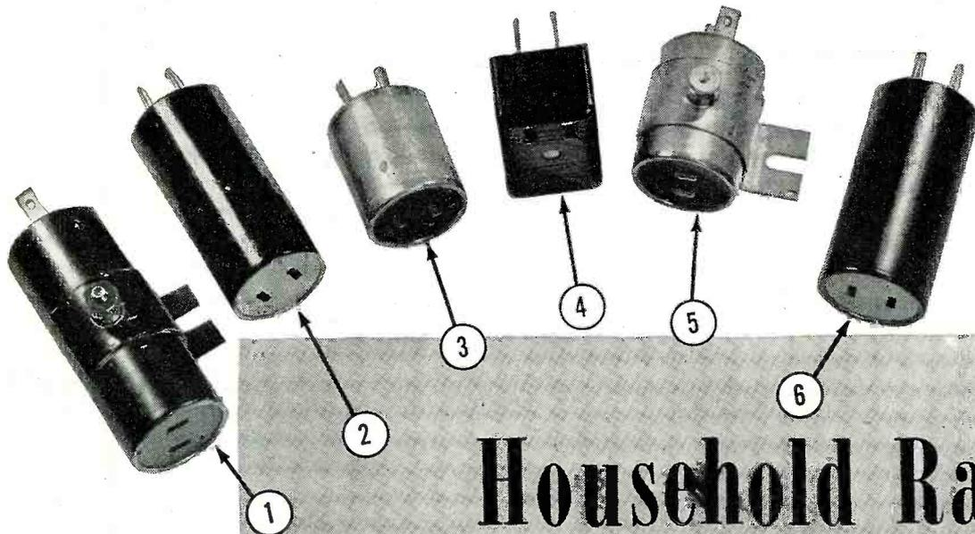
Fig. 1. Six plug-in type interference filters that were tested by the author. Nos. 1-6 tie in with the graphs shown in Figs. 3 and 4.
