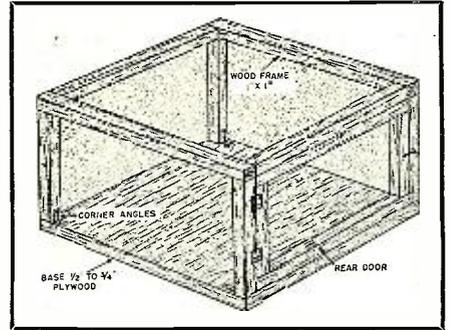
Fig. 7. A wooden framework completely covered on six sides with copper screening can be used to shield entire unit.
