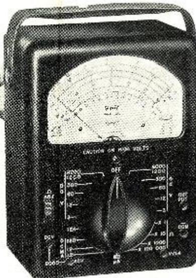
testers are very susceptible to accidental damage because it is very easy to forget to turn the selector switch to the desired function. If you want to check power line voltage, for instance, and have the switch on the 0-120 milliamperes position, you'll probably hear a quick "fffft" as you plug in the test leads. That sound represents your investment going up in smoke, literally. Sure, the meter can be repaired, but it will cost money.
