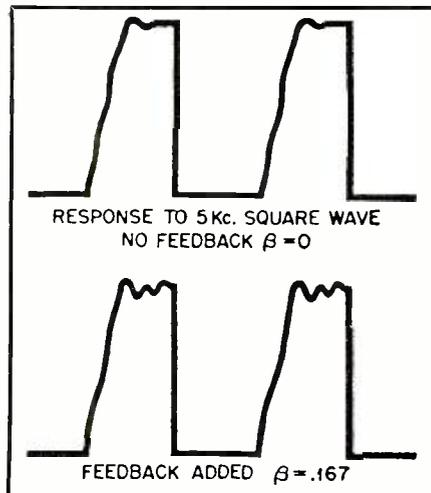
Fig. 7. Transient response measurements of an amplifier with and without feedback.
