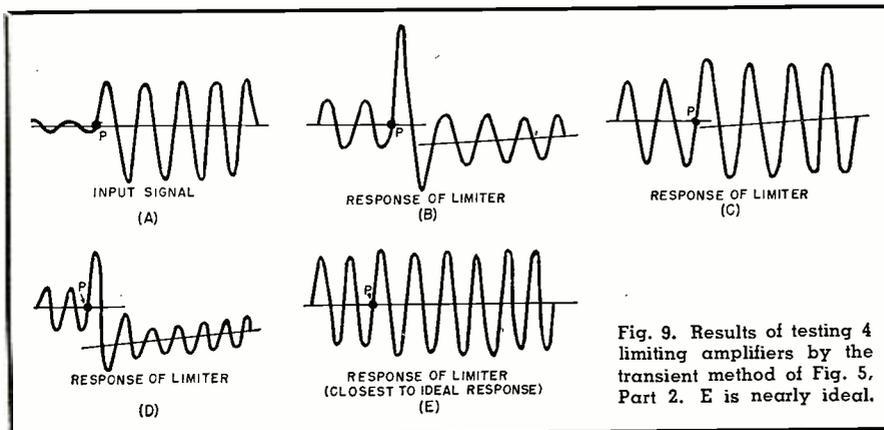
Fig. 9. Results of testing 4 limiting amplifiers by the transient method of Fig. 5, Part 2. E is nearly ideal.
