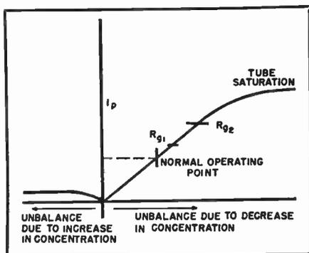
Fig. 4. Plate current of detecting tube.
