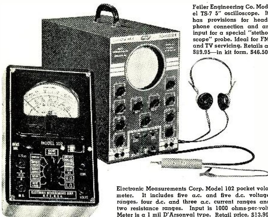
Feiler Engineering Co. Model TS-7 5" oscilloscope. It has provisions for headphone connection and an input for a special "stethoscope" probe. Ideal for FM and TV servicing. Retail at \$89.95—in kit form, \$46.50.
