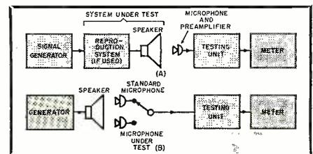
Fig. 5. Testing of reproduction systems involving direct sound pickup or reproduction. (A) Testing loudspeaker with standard calibrated microphone. (B) Testing sound pickup system by comparison with standard calibrated microphone.
