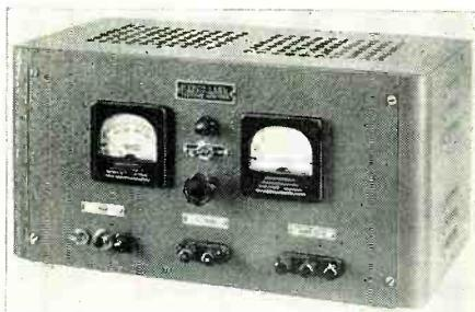
rents from 0 to 200 milliamperes, regulated; a.c. output is 6.3 volts at 6 amperes, unregulated.
