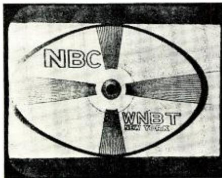
Fig. 5. Image possessing insufficient height.
