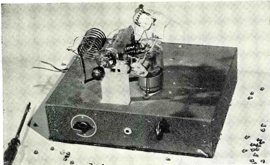
This is a 28 mc. 815 "breadboard" type with 56 mc. plate traps installed.
