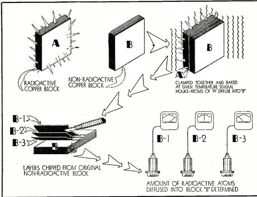
Fig. 1. Self-diffusion technique, imparting radioactivity to pieces of like material, then measuring chips for presence of radioactivity with Geiger-Mueller detectors.
