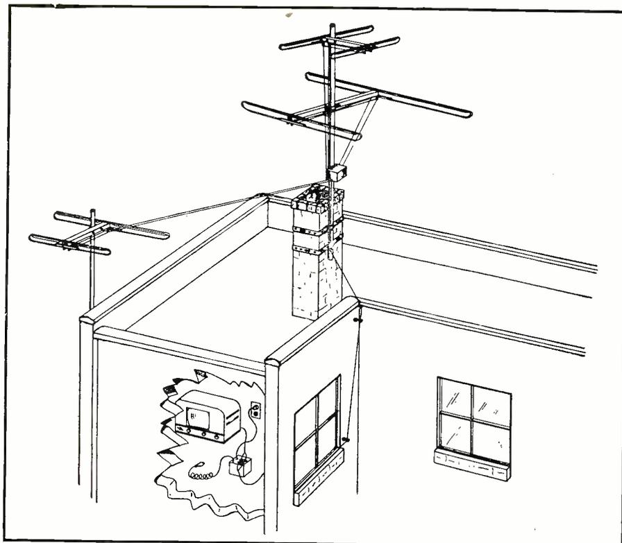
Fig. 2. Drawing of a complete Select-O-Vision installation.
