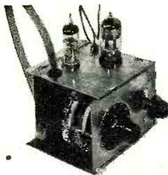
**NEW 13 CHANNEL TUNER** is a small compact unit with stage of R.F. Tunes all TV and 2FM channels. Made to conform with Telekit or any other TV set having video I.F. of 25.75 Mc. Complete with tubes, pre-wired, pre-aligned; only three connections to make. See your jobber, or write to us for information. Your cost, \$19.95.
