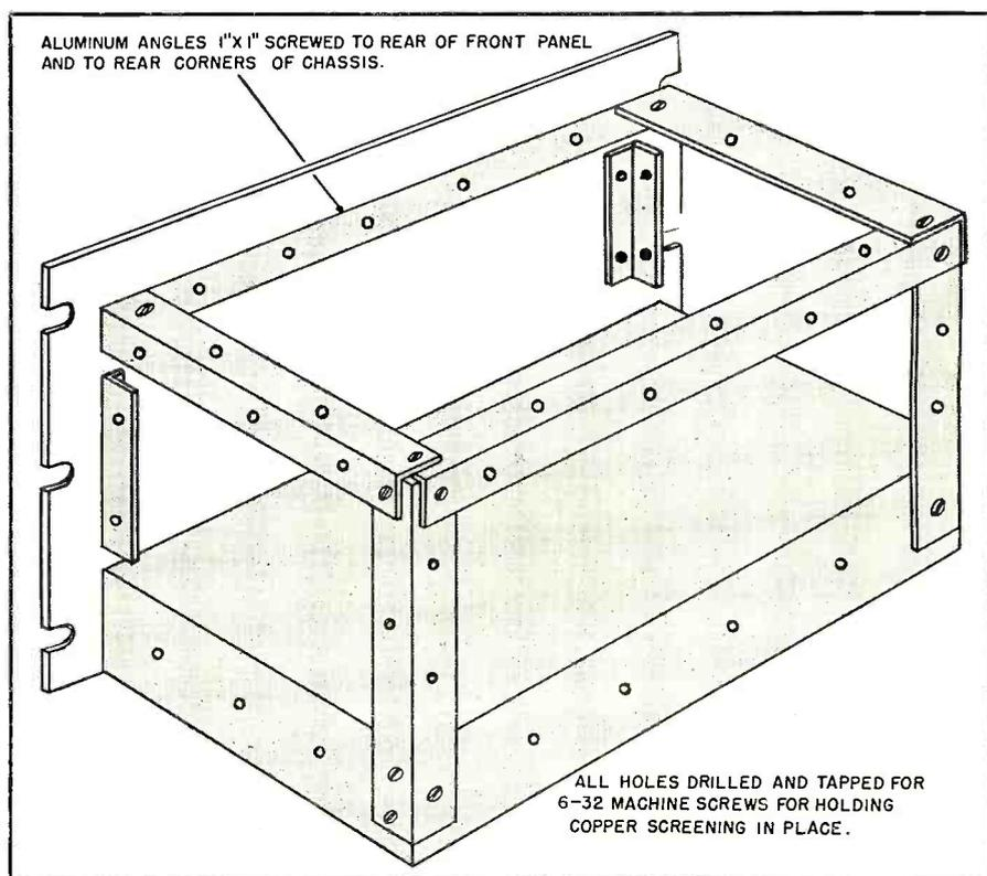
ALL HOLES DRILLED AND TAPPED FOR 6-32 MACHINE SCREWS FOR HOLDING COPPER SCREENING IN PLACE.
