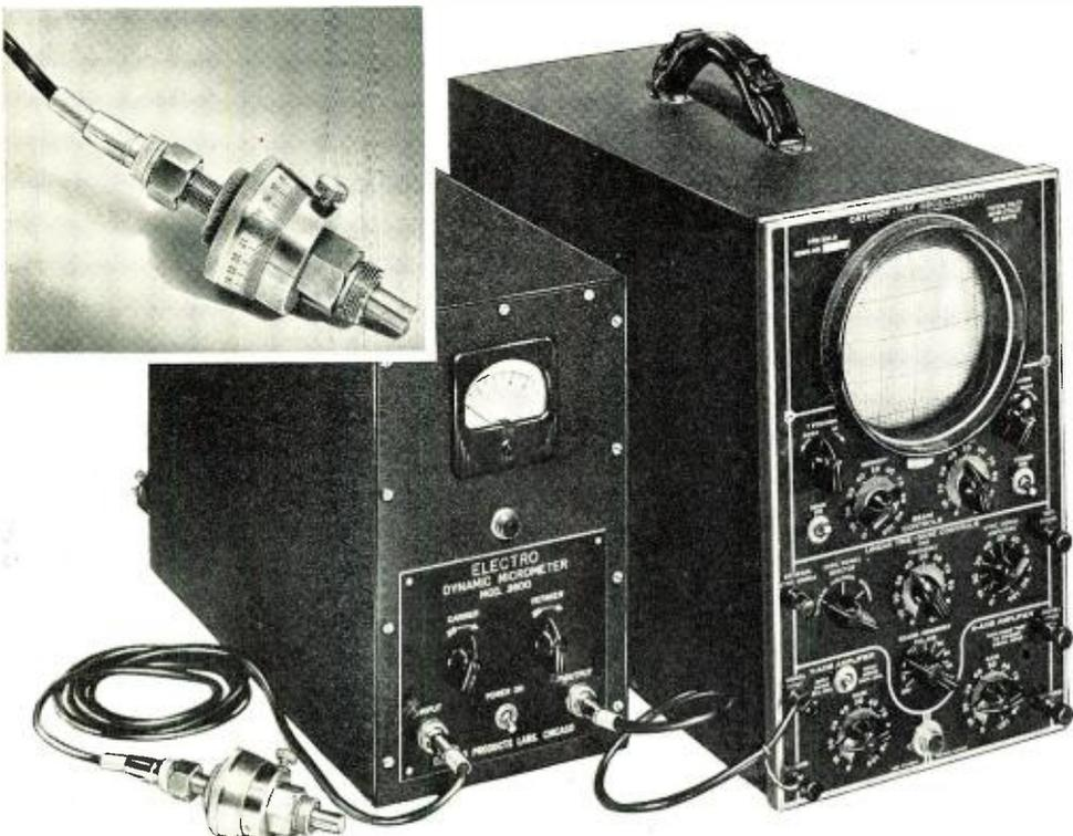
Fig. 1. The dynamic micrometer. Inset (upper left) shows a close-up of the micrometer sensing element.
