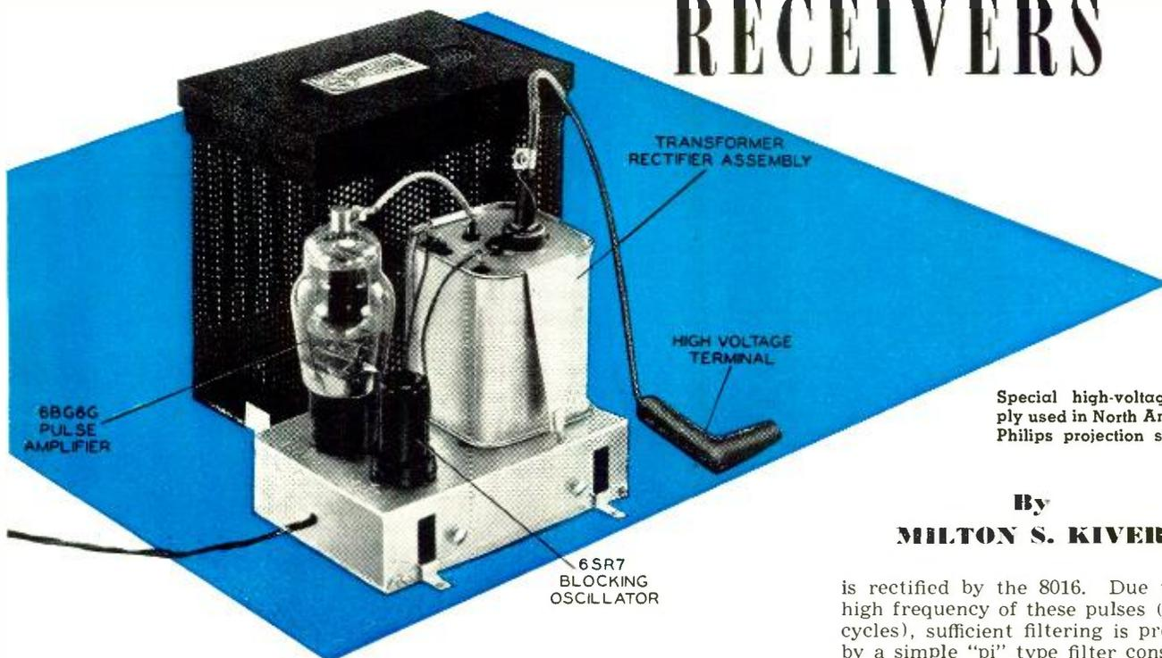
Special high-voltage supply used in North American Philips projection systems.
