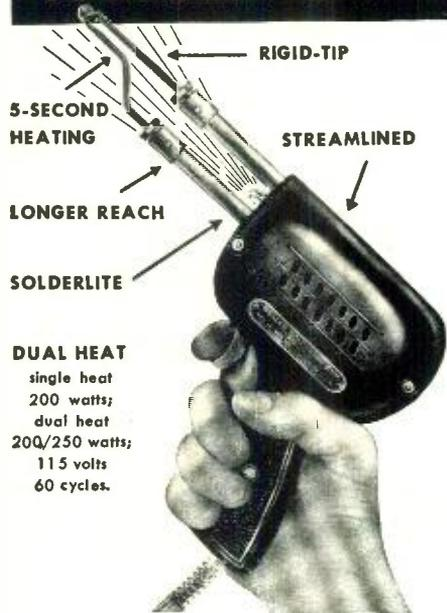
You'll save on tools and time with the new Weller Soldering Gun WD-250. Whether the job is rugged or delicate, your Weller Gun does it with the same ease and efficiency. Chisel-shaped RIGID-TIP provides more soldering area for faster heat transfer. New "over-and-under" terminal design gives bracing action to tip. Your Weller Gun is light-weight and compact, gets into the tightest spots.
