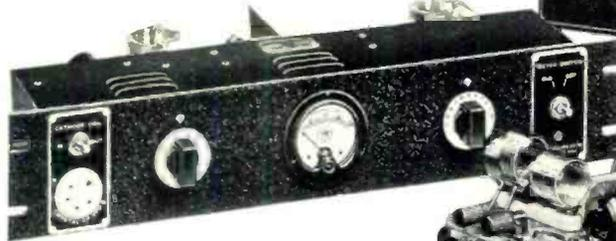
↑ A 50 watt transmitter-exciter unit by Millen. Requires an external power supply and features plug-in coils.
