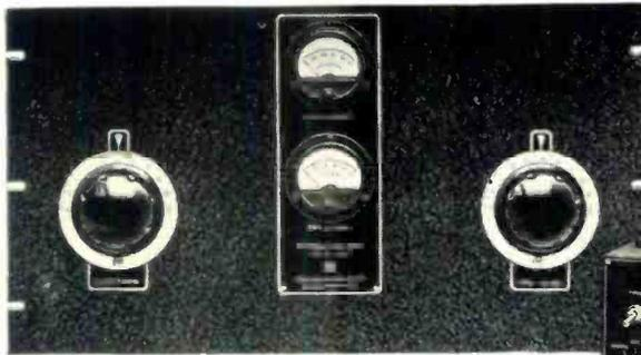
Millen bandswitching v.f.o., featuring full → bandspread on all bands from 80 to 10 meters.
