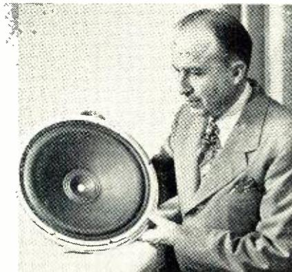
from approximately the same conical surface, the two-cone-sections are mounted in a single housing.
