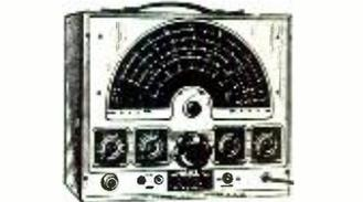
Complete FM-TV frequency coverage from 2-227 MC on 3 bands. Sweep width 500 KC to 10 MC. Dial calibrated directly in frequency. Maximum output 500,000 microvolts. Built-in power line filter. Generator output can be used either FM or pure RF. 105-125 volts, 50/60 cycles AC. Steel cabinet finished in gray wrinkle enamel. Shpg. Wt. 16 lbs.
