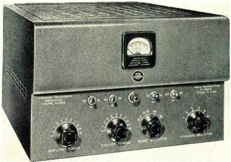
The Stancor ST-202-A c.w. transmitter kit will handle an input of 125 watts.
