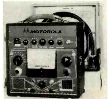
Fig. 6. Motorola test set plugs into this maker's receivers for quick checks.
