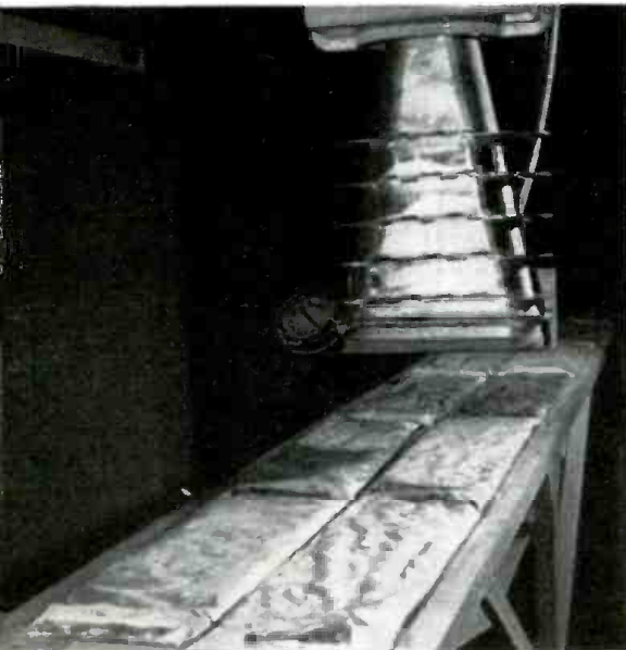
▲ Fig. 1. Cranberries are passed under swept beam of a super voltage electron beam generator by conveyor belt and subjected to electron bombardment and sterilization.
