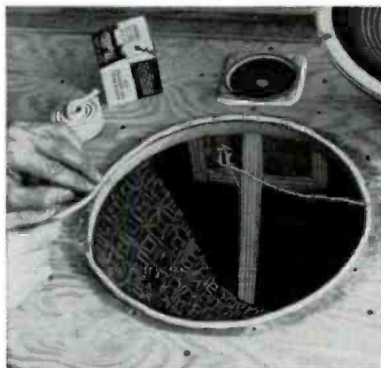
The method of making the seal required for the woofer is illustrated above.
