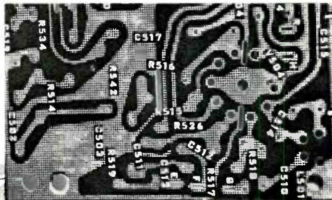
Fig. 3. (Left) Part of a printed-board diagram from the manufacturer's service data, to assist in component location.
