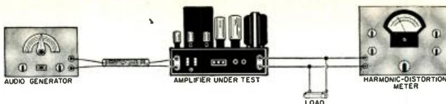
Fig. 2. The basic setup that is employed in measuring total harmonic distortion.
