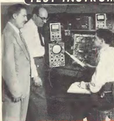
In the Majestic design laboratories, Frank J. Dieli and assistant, Paul Smith, discuss with Harry R. Ashley, some important prototype-circuit measurements just taken with the 425 Oscilloscope, #221 VTVM and #HVP-1 HV Probe.
