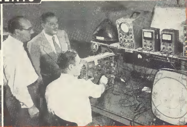
Frank J. Dieli, Majestic's Chief Engineer, and Harry R. Ashley, President of EICO, inspecting the use of the EICO Model 425 5" Push-Pull Oscilloscope, Model 221 Vacuum Tube Voltmeter and Model HVP-1 High Voltage Probe of the important Final Test Position on the Majestic Television production lines.
