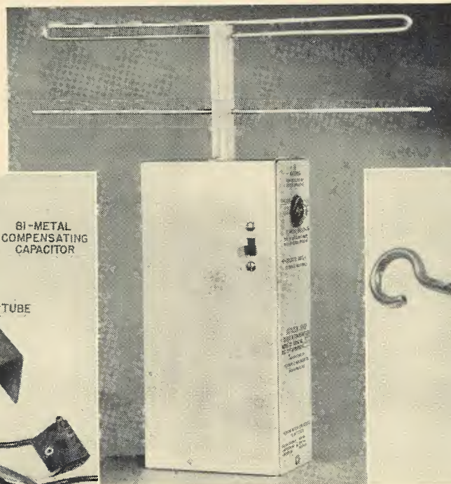
Fig. 4. Over-all view of transmitter with antenna. The entire radio-control unit weighs less than four lbs. including batteries. →
