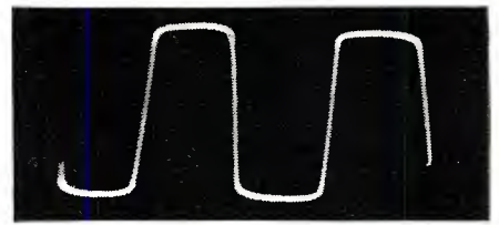
Fig. 3. Output waveform of the calibrator, fed to scope's vertical input.
