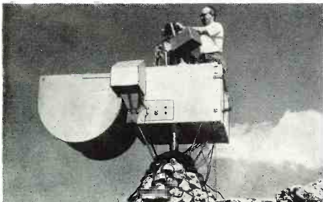
Sensitive photoelectric photometer used to observe airglow.
