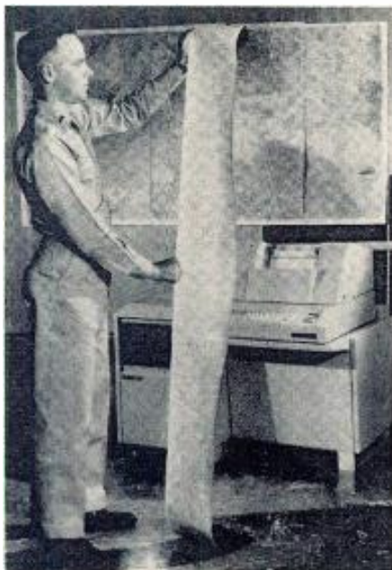
Officer is holding 3000-word message that has been typed by new Army teleprinter in just one minute flat.
