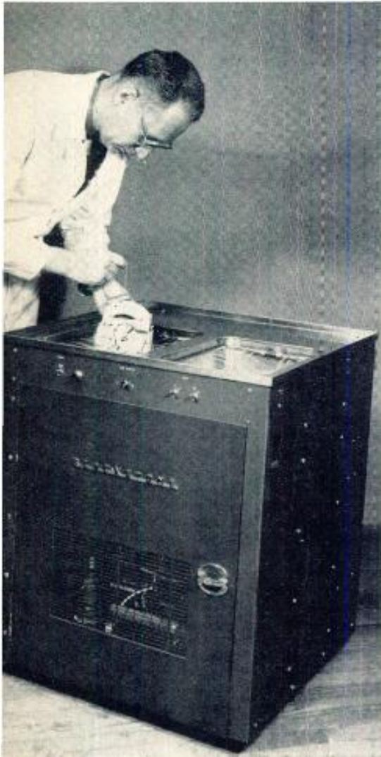
Fully assembled parking meter is being cleaned in the ultrasonic bath at the left.
