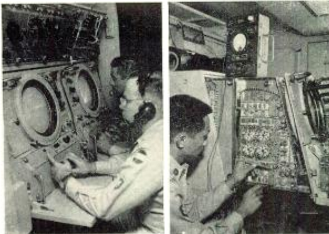
Scope at extreme left shows range and bearing data, while other display shows altitude. At right, entire indicator console has been pulled out on rollers to provide easy servicing.
