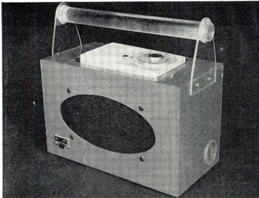
The personal portable fits neatly into a recessed opening in the carrying case housing the added amplifier and loudspeaker.
