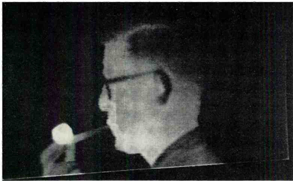
Fig. 1. Infrared photo (thermograph) taken in total darkness. In this view black areas are at a temperature of 75 degrees F or colder, and white areas are at 133 degrees or hotter. Note that the pipe bowl is the hottest object in the photograph.
