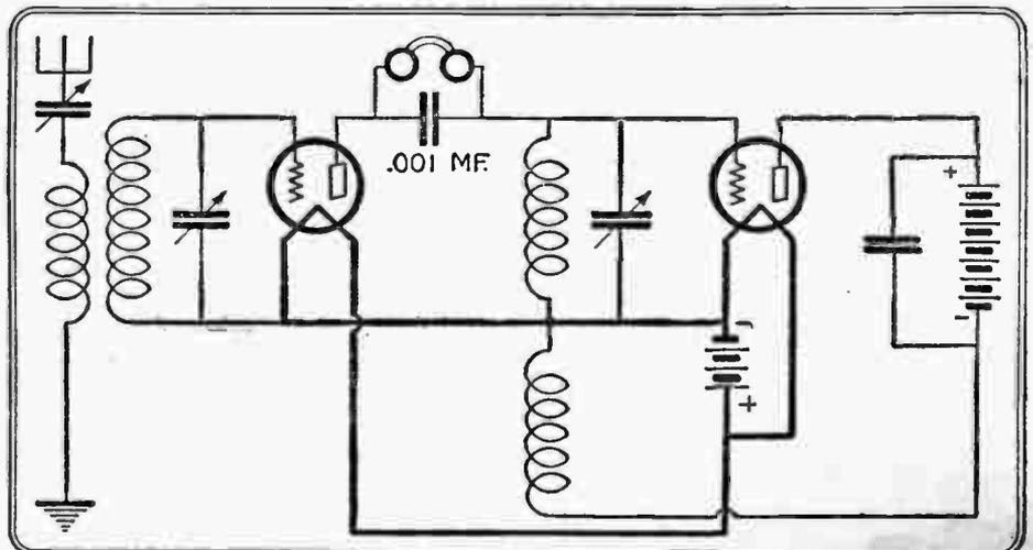
(399-C). The fundamental principle of the Ultradyne receiver, showing the first detector and oscillator circuit employing the efficient modulation system. This method is a radical departure from the conventional, and results in a receiver of remarkable efficiency.
