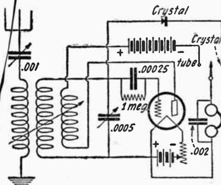
(56) A Crystal or a Tube May Be Used as the Detector in This Circuit by Means of the Single Pole, Double Throw Switch.
