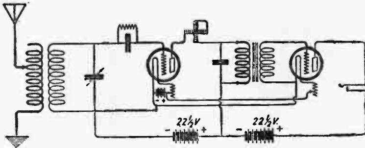
Q. 1. Please publish a diagram of a single-stage amplifier using a Peerless coil. A zinc shield is used. How can extreme body capacity be eliminated?
