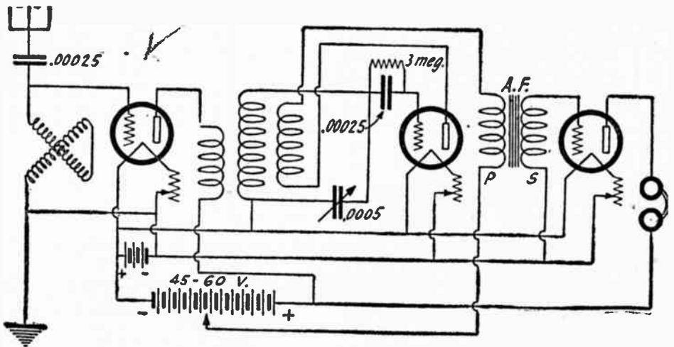
(52) Regeneration Can Be Used in Conjunction with a Radio Frequency Amplifier if This Circuit is Used. Details Are Given in the Text.
