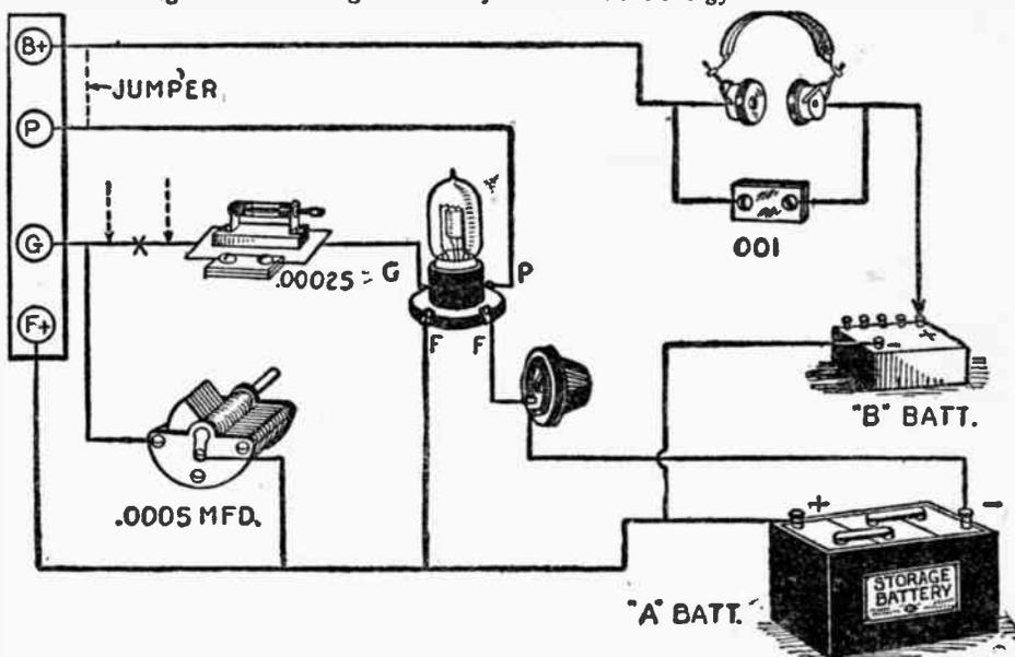
(111) This picture diagram of a tube unit and the diagram of one of the coil units shown above, should enable anyone to construct a very efficient 1-tube receiver. The completed set may be later enlarged to include audio frequency amplification if the owner desires to operate a loud speaker.
