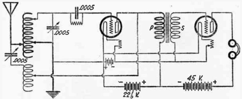
(109) Audio Frequency Amplification May Be Added to the Reinartz Circuit By Following This Diagram.
