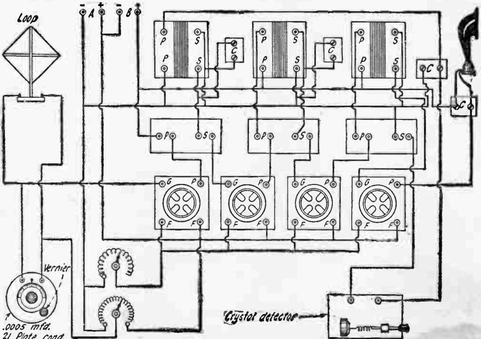
(219) Circuit Diagram of the Acme Four-Tube Reflex Receiver Using Three Radio and Three Audio Frequency Transformers. Further Details Are Given in the Text.
