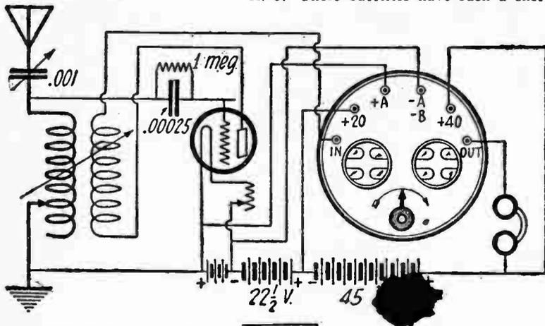
(4) This Shows How the Atwater-Kent Two-Stage Amplifying Unit is Connected to a Single-Circuit Receiver.
