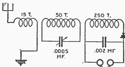
(135) A crystal receiver circuit designed for selectivity. It is also the height of simplicity.
