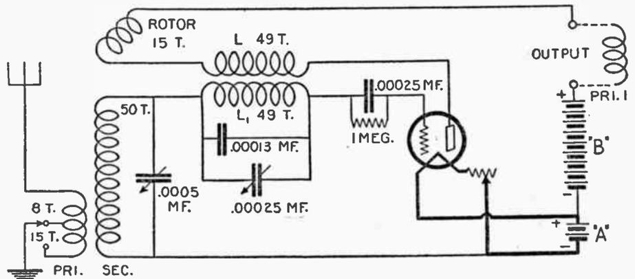
(196) The O'Connor frequency changer, which may be used in connection with any receiver.
