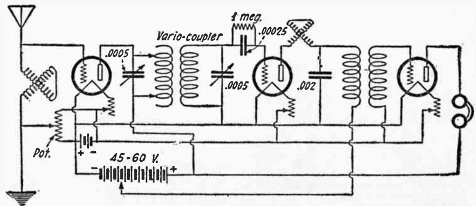
(13) Here is shown the best method of using one stage of R.F. amplification with a standard regenerative receiver.
