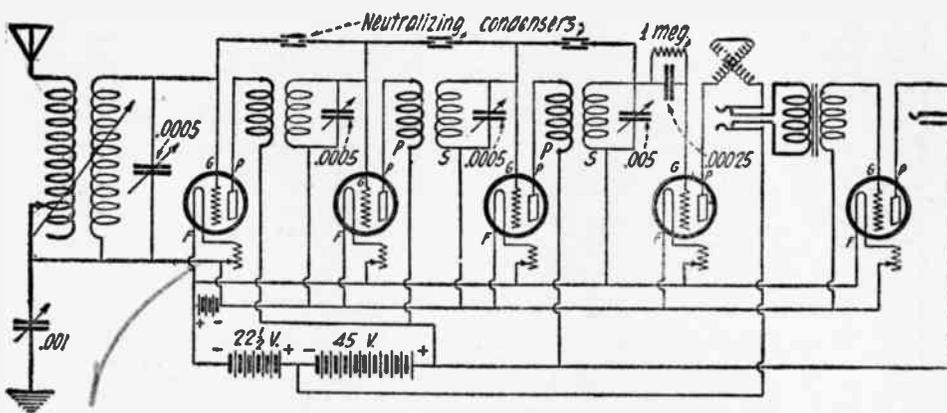
(110) The Neutrodyne Receiver, Using Three Stages of Tuned R. F. Amplification. No Potentiometer is Used in This Circuit, the Secondaries of the Transformers Being Connected Directly to the Negative Side of the "A" Battery.
