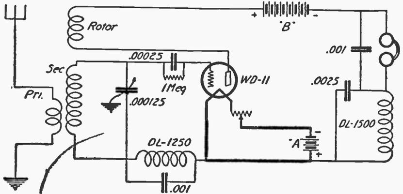
(104) Super-regeneration, or regeneration, at short wave-lengths? By a slight change, the experimenter has either available, at will. We will welcome reports, addressed to the editor, on reception conditions in various parts of the world, at short wave-lengths.
