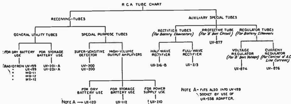
(258) This chart may be used to determine the best tube for receivers, both plain and those employing various methods of amplification, or using dry cells in place of storage batteries.
