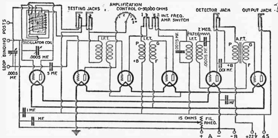
(398-A). The original circuit used by the Western Electric Company in their type 6004-C radio receiving outfit. The oscillator coil design and connections are included in the diagram; the two 48-turn windings being placed on a 2-inch tube; the 40-turn winding on a 1-inch tube mounted within the 2-inch tube coil.
