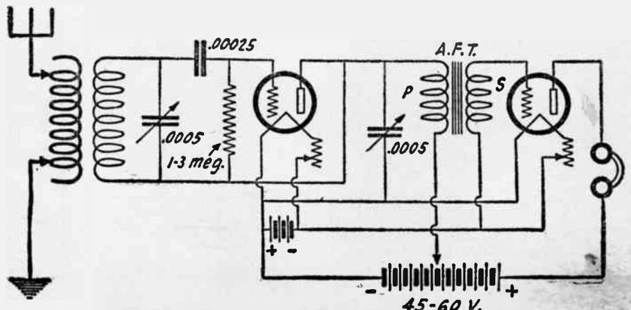
(47) Good Results Will Be Had With the Well Known Ultra Audion. The .0005 mfd. Variable Condenser Connected from the Plate to the Filament of the Detector Tube Controls the Regeneration.
