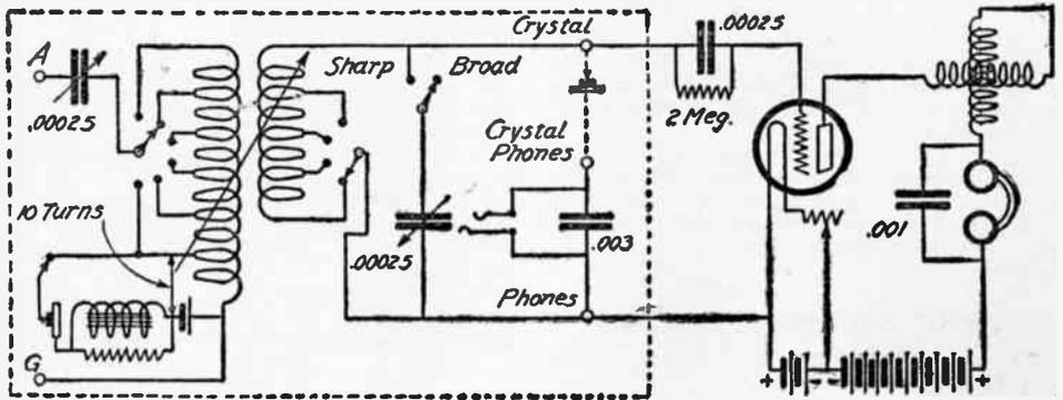
(17) A Signal Corps crystal set may be changed into an efficient tube unit, as shown here.
