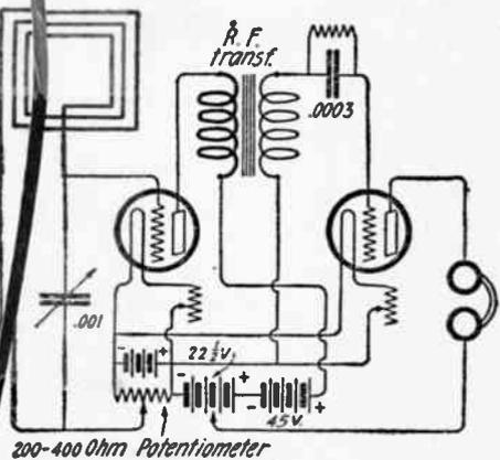
(18) A Two Tube Loop Antenna Set with one Stage of Radio Frequency Amplification. Variation of Wavelengths is Accomplished by the Variable Condenser.
