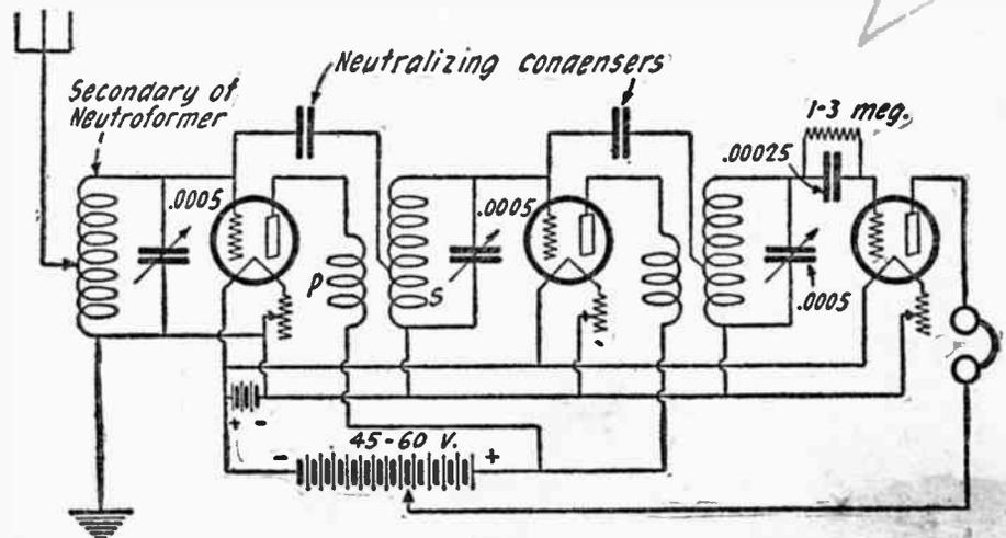
(60) The Neutrodyne Circuit Using Two Stages of Radio Frequency. The Secondary of the First Neutrodyne is Used as the Tuner.
