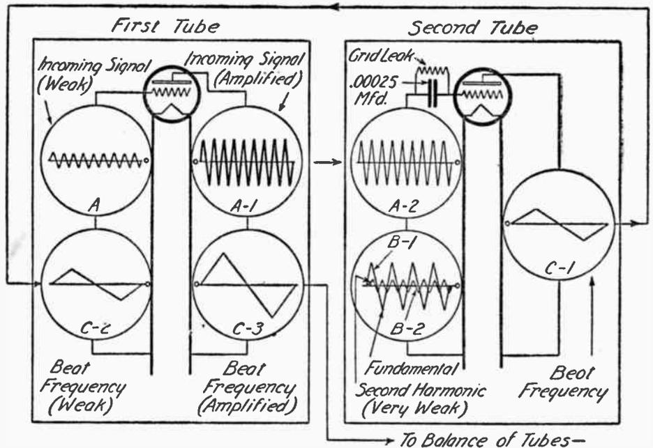
(189-A) The Second-Harmonic Super-Heterodyne principle of operation, graphically shown. The accompanying text explains the system in considerable detail.
