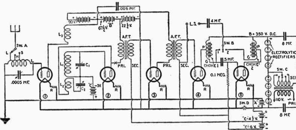
(323) An unusual circuit employing the use of electrolytic rectifiers to supply B voltage for the plates of the last two amplifier tubes. (See page 71).
