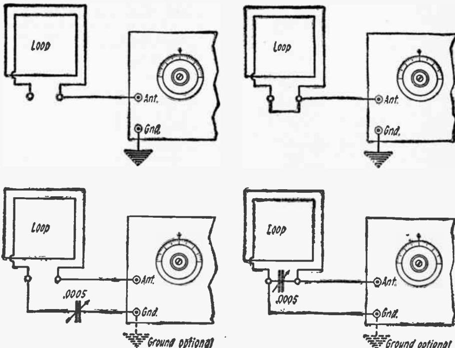
(130) Showing a number of different methods of employing a loop aerial with a Neutrodyne receiver. The use of a ground connection will reduce the directional effect of the loop aerial considerably.
