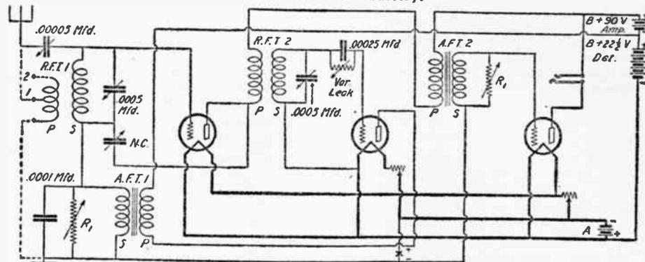
(200) The new Harkness reflex circuit, neutralized. This set will be found extremely selective if apparatus of good quality is used. Any type of tube may be used if sockets and rheostats are changed accordingly.
