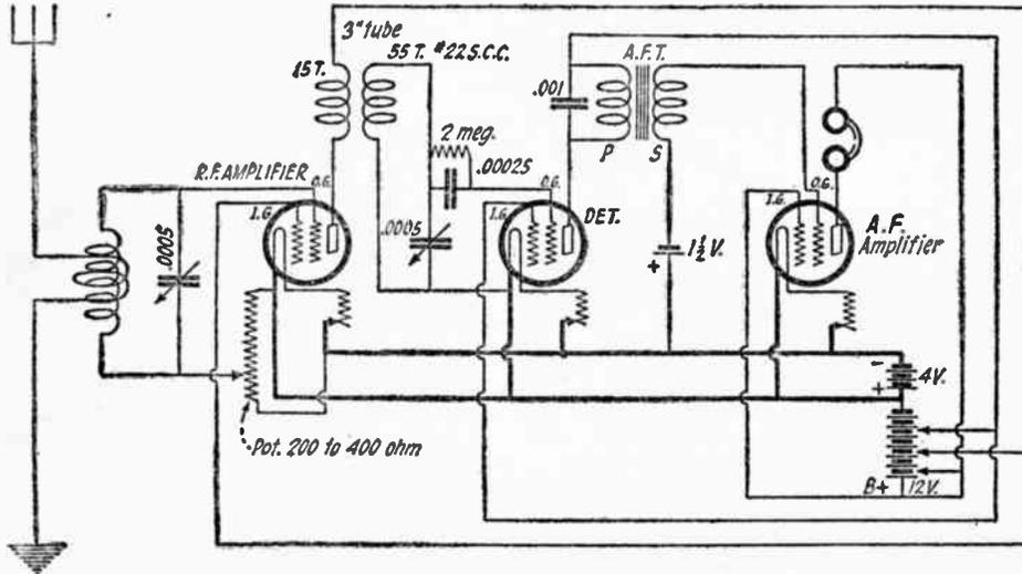
(102) The use of double grid tubes as radio frequency amplifiers, detectors and audio frequency amplifiers is clearly shown. Solodyne tubes might work in this circuit.
