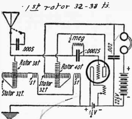
(245) Diagram of the Aeriola, Sr. Receiver. Two Variometers Are Used, One as the Tuning Unit and the Other in the Plate Circuit.
