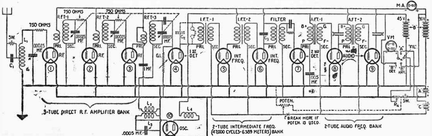
(206) The Experimenters' Information Service Navy Model C-10 super-heterodyne designed for a wave-length range from 600 meters down to 50 meters, the band being covered through the expedient of interchangeable coils. Blueprints are not available.
