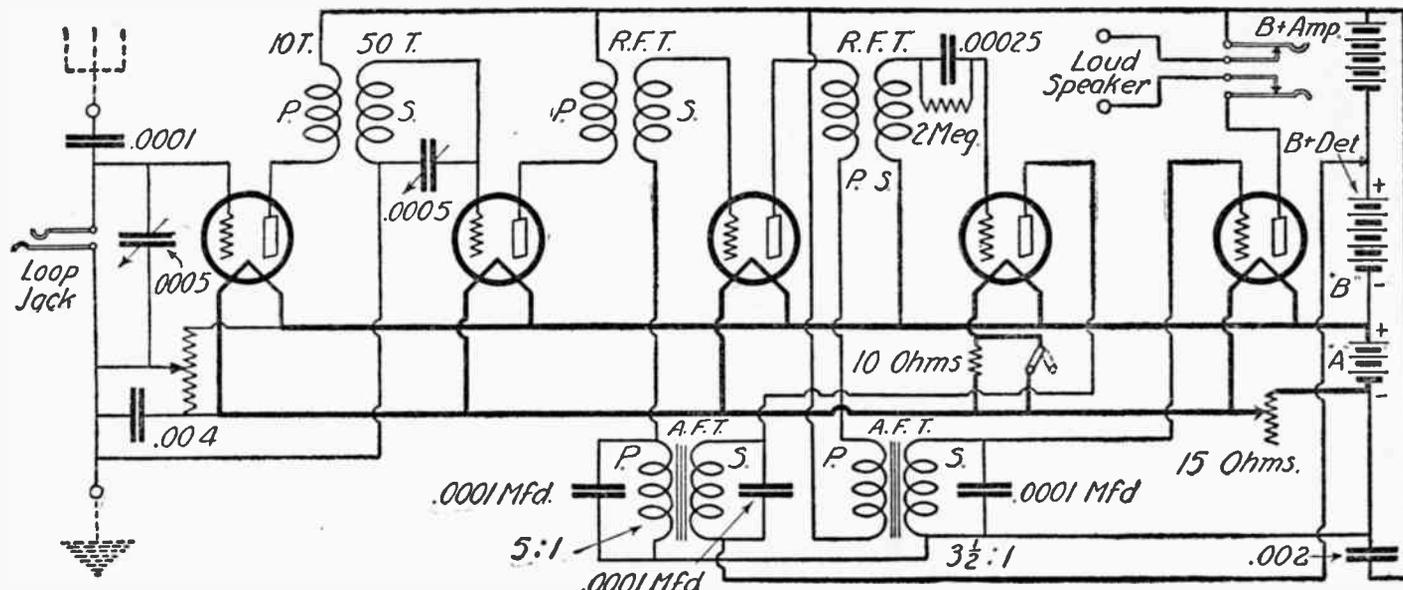
(197) The DeForest D-17 Reflex Loop Receiver. There have been a great many requests for this modern reflex circuit. The usual crystal detector has been replaced by a tube detector.
