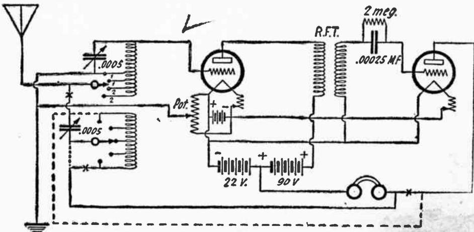
(34) Two methods of adding regeneration to the Reinarts circuit are shown here. If the dotted lines are followed, regeneration is obtained by the tickler feedback method.
