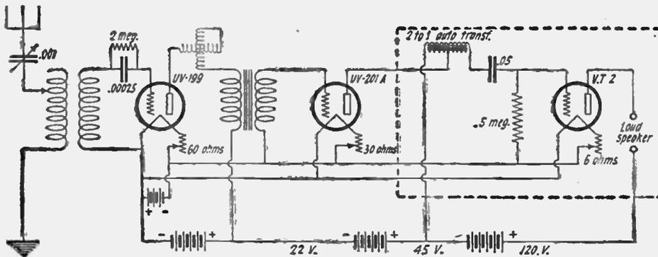
(39) A regenerative circuit with a two-stage audio frequency amplifier. The second stage is a power amplifier and employs an auto transformer. A high "B" battery voltage is essential.
