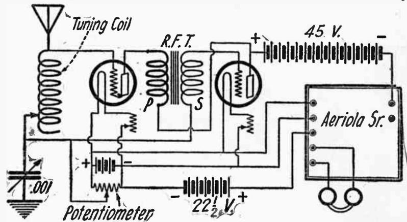
detector and two stages of audio frequency.
