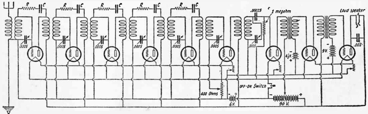
(233) This Super-Plodyne illustrates the Ferrand system for controlling the oscillations in radio frequency amplifiers, extended to include six stages of radio frequency amplification. Every stage must be carefully balanced. All the variable condensers are geared to one dial.
