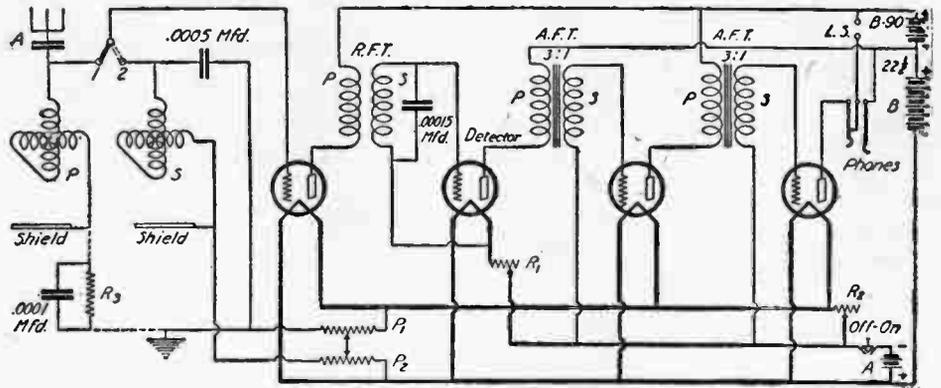
(217) The Amrad "Inductrole." Variometers are employed in an efficient manner. The receiver is so designed that grid current leakage through the set is just sufficient to prevent the first tube from "blocking." The commercial receiver reproduces with excellent fidelity.
