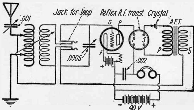
(240) Remarkable Results Are Claimed for the "Erla Duo-Reflex" Circuit, Shown Here. Only One Tube is Used for Two Stages of Amplification.
