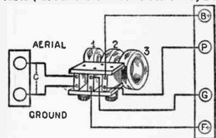
(111-C) The "3-coil honeycomb" regenerative unit. The standard way of receiving long-wave stations.
