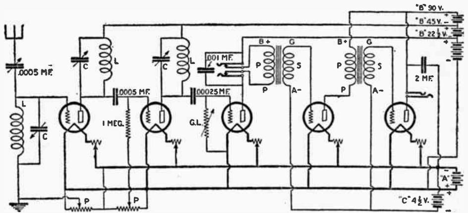
(89) Tuned Impedance. The standard schematic circuit for a receiver using "tuned impedance" coupling. Each tuned unit, when adjusted for a given signal, "rejects" that signal, causing the signal to charge the blocking condenser and, in turn, operate the grid of the amplifier tube. Undesired signals are "accepted" and do not operate the amplifier tubes. The circuit shown is very selective.
