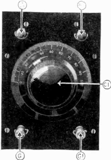
Fig. 11. A front view of the wavetraps, the circuit of which is shown in Fig. 4 A. Note that there are two aerial and two ground posts. Photos courtesy of X-L Radio Laboratories.
