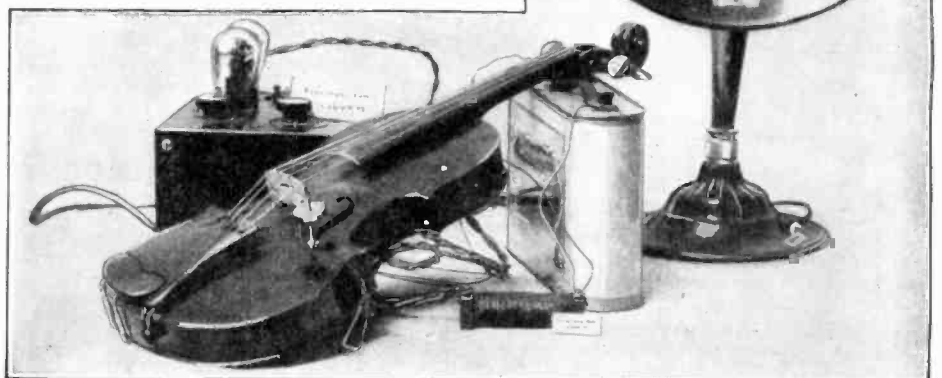
The complete outfit for making a violin play with enormous volume. Above is shown a transmitter button of another type, which can be used instead of that shown.
