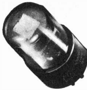
The FM tuning indicators shown here include the 6E5 and the 6AL7 tuning eye tubes along with a space-saving, side-indicating type tuning meter.
