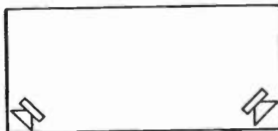
Fig. 8. Here is the Ampex method of housing two stereo speakers within one cabinet.
