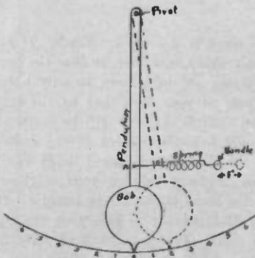
Fig. 3. A Case of Tight Coupling
