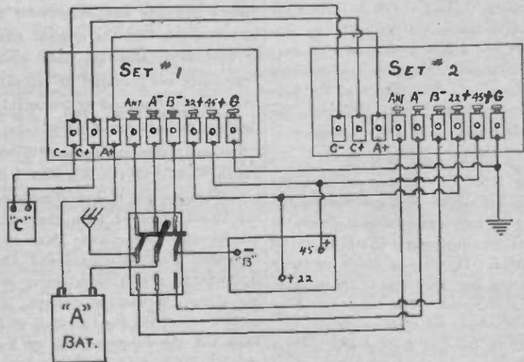
Fig. 2. Simplified Hook-up—3-Pole Switch
