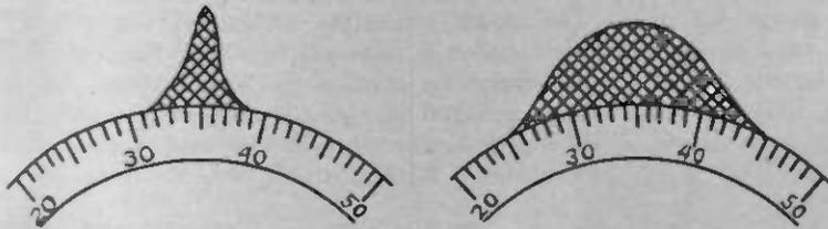
Fig. 5. The Shaded Area Shows Loudness of a Station As the Dial is Turned. The Sharp Tuning is at Left
