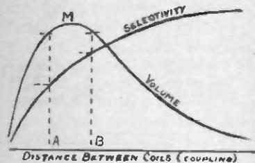
Fig. 4. Selectivity But not Volume Increases with Distance of Coils
