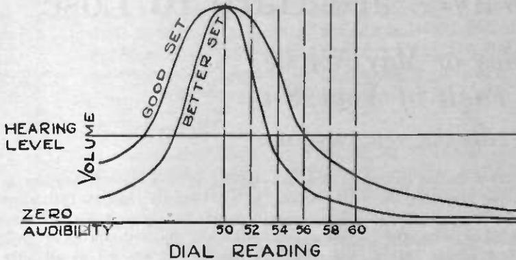
Fig. 3. The Better Set is Much Softer When Thrown Slightly Out of Tune. At 53 it Disappears
