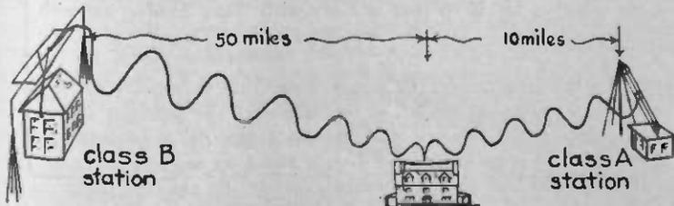
Fig. 1. A Big "B" Station Far Away May Give Same Wave as Small "A" Sender Near By
