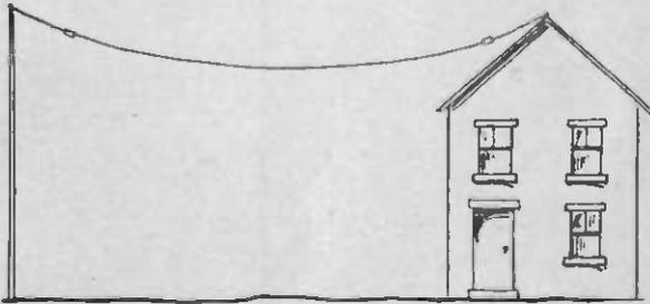
Fig. 2. With This Construction Your Signals Will Sometimes Fade
