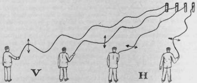
Fig. 4. Two Men Shake the Clothes Lines Up and Down (Vertical), the Others Back and Forth (Horizontal)
