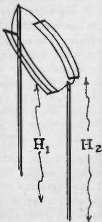
Fig. 7. The Principle of Wave Shift with Swinging Aerial
