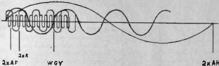
Fig. 1. Four Waves, All Going at Once, Come from the Transmitters of Schenectady. Their Relative Frequency and Length Are Shown Here
