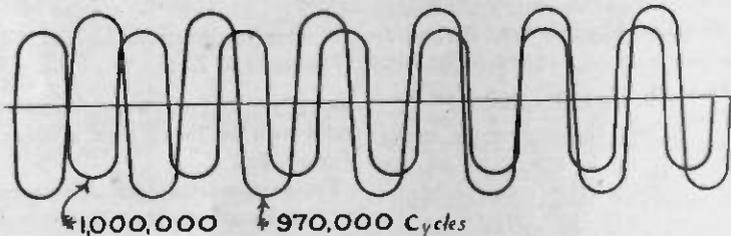
Fig. 8. Two Waves of Almost the Same Speed Will Give Very Broad Tuning if From Same Station
