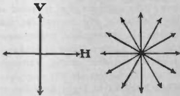
Fig. 5. Polarized Waves May be Horizontal or Vertical, but Most Waves Are in All Directions.
