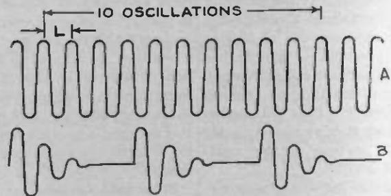
Fig. 4. Tuning for 10 Waves is Easy with Tube Sender, but with Spark It Can't Be Done
