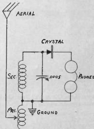
Fig. 2. (Reprint from First Part) Hook-up of Crystal Set
