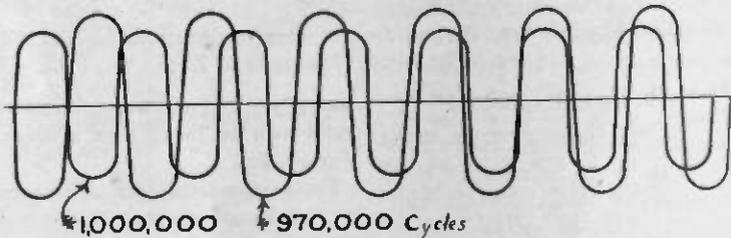
Fig. 8. Two Waves of Almost the Same Speed Will Give Very Broad Tuning if From Same Station
