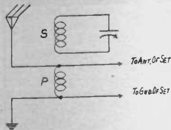
Fig. 6. Parallel Connection of Trap
