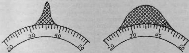
Fig. 5. The Shaded Area Shows Loudness of a Station As the Dial is Turned. The Sharp Tuning is at Left
