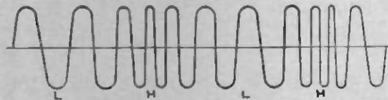
Fig. 6. A Swinging Aerial May Cause a Wave to Change its Speed as Shown
