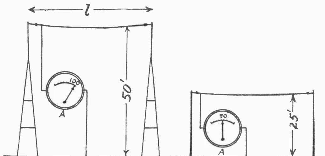
Fig. 2. The Electric Field on Signal Strength is Same at Both Antennas, Although of Different Heights.
