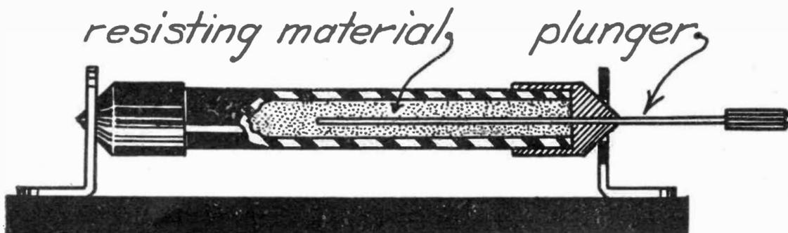
Fig. 6. The Basic Principle of Most Variable Leaks
