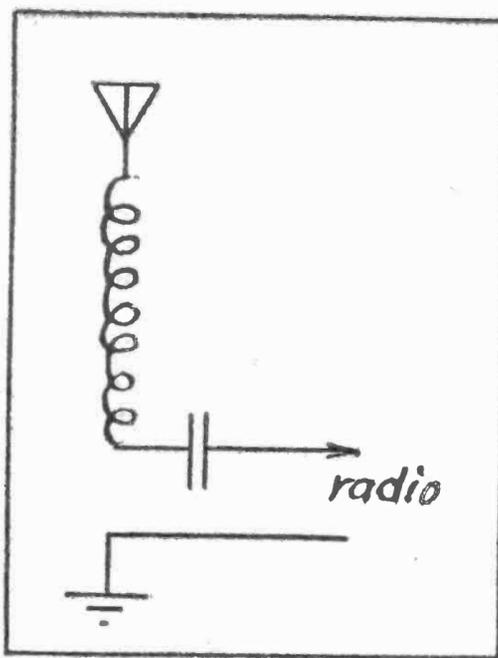
Fig. 3. This Acceptor Circuit Allows Only the Wanted Signal Through.
