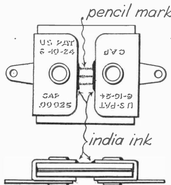
Fig. 9. The Home-made Leak. Don't Omit the India Ink
