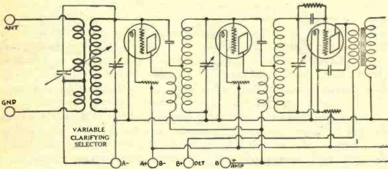
Fig. 2. Using Special Coupler is Easy in a 3 to 5-Tube Set.
