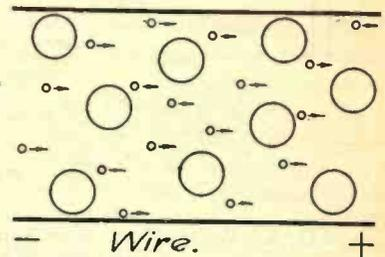
Fig. 5. A Copper Wire Conducts Current in This Way
