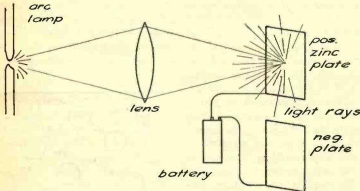
Fig. 6. When Light from Lamp Strikes Zinc Plate it Liberates Electrons Which Make Current
