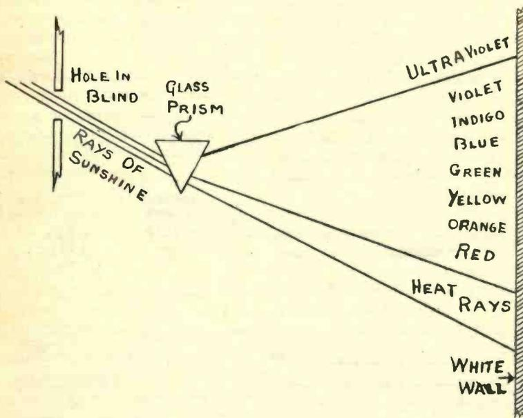
Fig. 3. How a Beam of Sunlight May be Broken Into the Colors of the Rainbow or Spectrum
