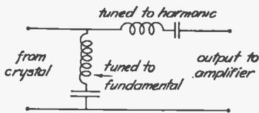
Fig. 5. Here is the Filter that Strains Off the Scum
