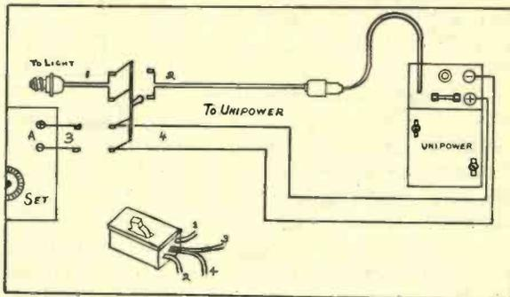
Fig. 4. The Switch Connects Either the Set for Listening or Battery for Charging.
