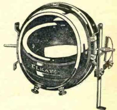
Fig. 1. This Special Coupler Combines a Small Condenser on Same Shaft.
