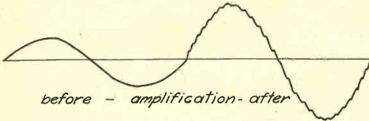
Fig. 3. Amplification Sometimes Brings Out Noise Which Was Not Noticed Before.
