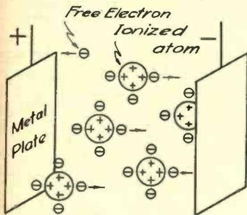
Fig. 1. When Salts Are Dissolved in Water, They Break Up
