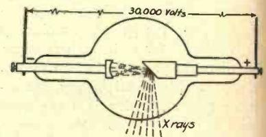
Fig. 7. Principle of an X-ray Tube. Note Electrons.
