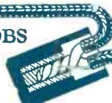
An Insulating Cap with a split screw that bites twisted wire ends.
