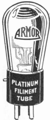
The ARMOR tube has—high filament emission—pure tone reproduction—long efficient life. It is non-microphonic—filament, grid and plate anchored in place, impossible to get out of alignment. Used in electric operated sets, the ARMOR tube has a distinct advantage over other tubes, as the filament emission is constant over a wide range of line voltage fluctuation.
