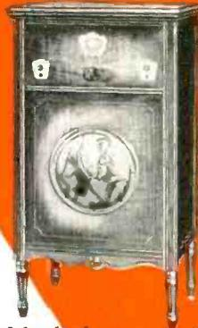
Console Model 520. Six tube, single dial vernier control. Selected walnut veneer cabinet with lustrous finish. Ample space for all batteries.
