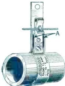
The Amoroso Radio Clamp is made of copper with a clip of nicked brass. The flanges are bent so as to give added strength and prevent the clip from turning. An exclusive feature. Ask about these clamps.
