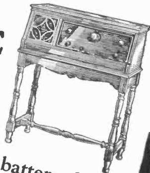
When it comes to battery elimination, this year's Day-Fan line has the world beaten. This AC Tube set needs no batteries—plug it into the light socket and the radio of the nation is at your finger tips. Supplied also in more elaborate cabinets (Day Royal and Day-Mar).
