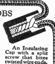
An Insulating Cap with a split screw that bites twisted wire ends.
