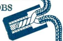
An Insulating Cap with a split screw that bites twisted wire ends.
