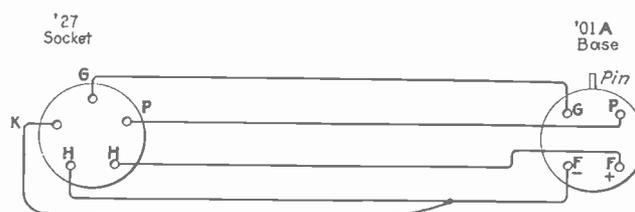
A.C. tube test circuit
