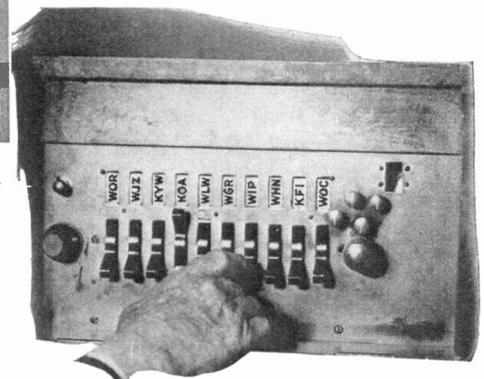
*(Right) The newest method of tuning—press a button and the station comes in automatically.*
