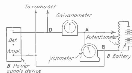
Fig. 3—Diagram for potentiometer method of measuring voltages of B-power units
