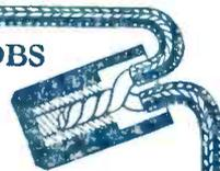
An Insulating Cap with a split screw that bites twisted wire ends.
