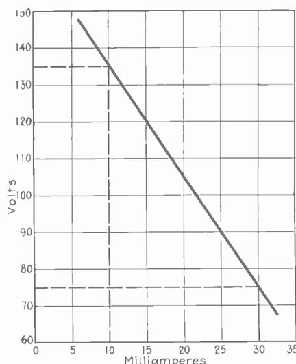
Fig. 1—Regulation curve of a B-power supply device
