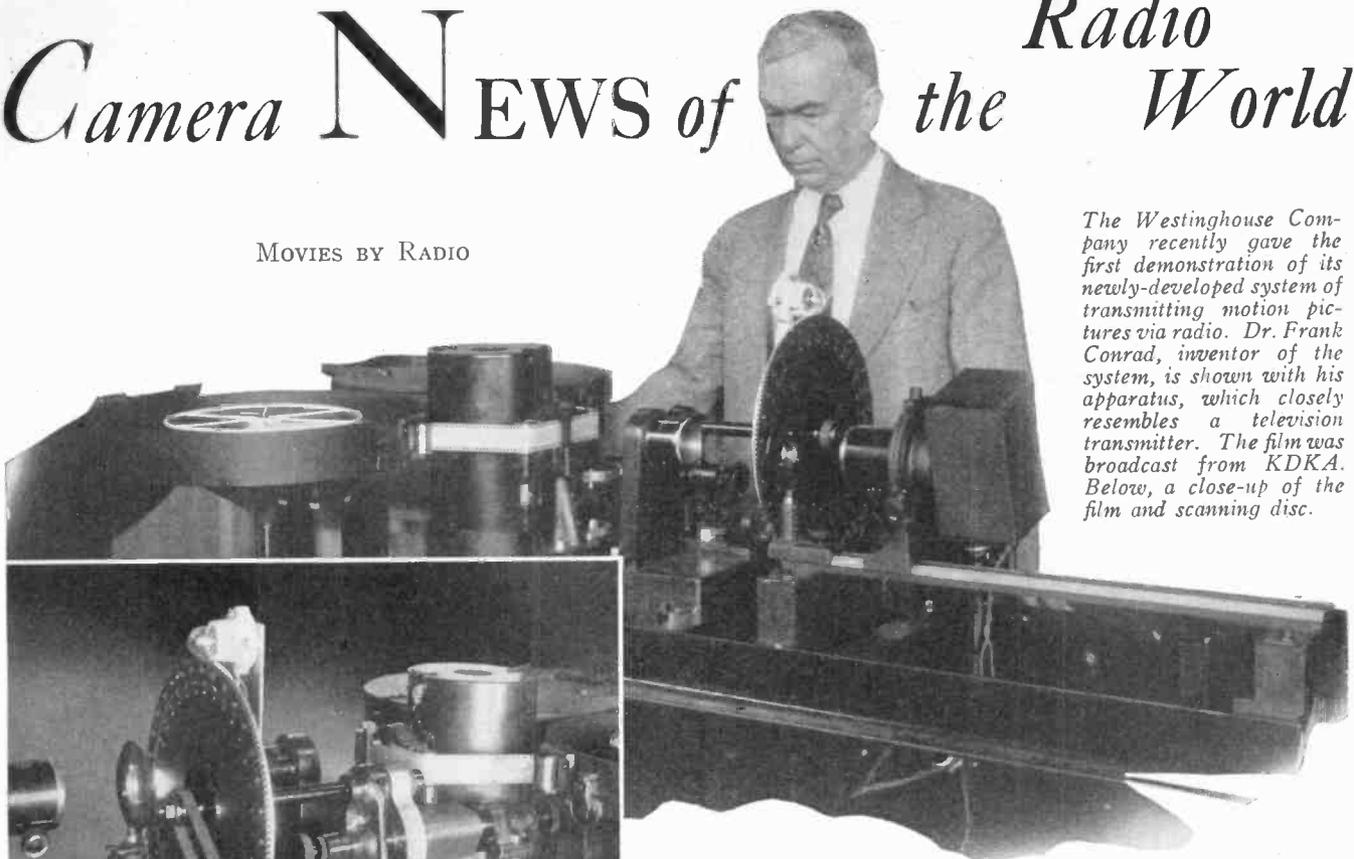
The Westinghouse Company recently gave the first demonstration of its newly-developed system of transmitting motion pictures via radio. Dr. Frank Conrad, inventor of the system, is shown with his apparatus, which closely resembles a television transmitter. The film was broadcast from KDKA. Below, a close-up of the film and scanning disc.
