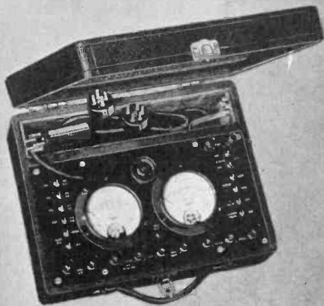
The Jewell No. 210 is the first tube tester to give direct readings, thereby eliminating mental arithmetic. It provides for variations in line from 100 to 130 volts. Tests all tubes. A 100 milliamperes scale is provided for rectifier tubes. Gives individual reading of each plate of double wave rectifier tubes. Operates from A.C. service line.
