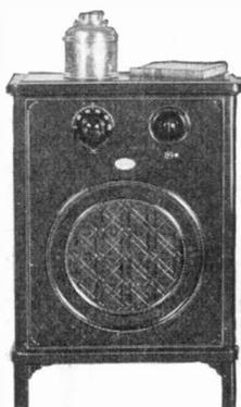
MODEL 53. New, compact, all-in-one set with Atwater Kent Electro-Dynamic speaker. Not much higher than your knee! Makes a beautiful little table for lamp or books — and becomes a musical instrument at the snap of the switch. Full-vision Dial. Requires 7 A. C. tubes and 1 rectifying tube. Without tubes, \$117.
