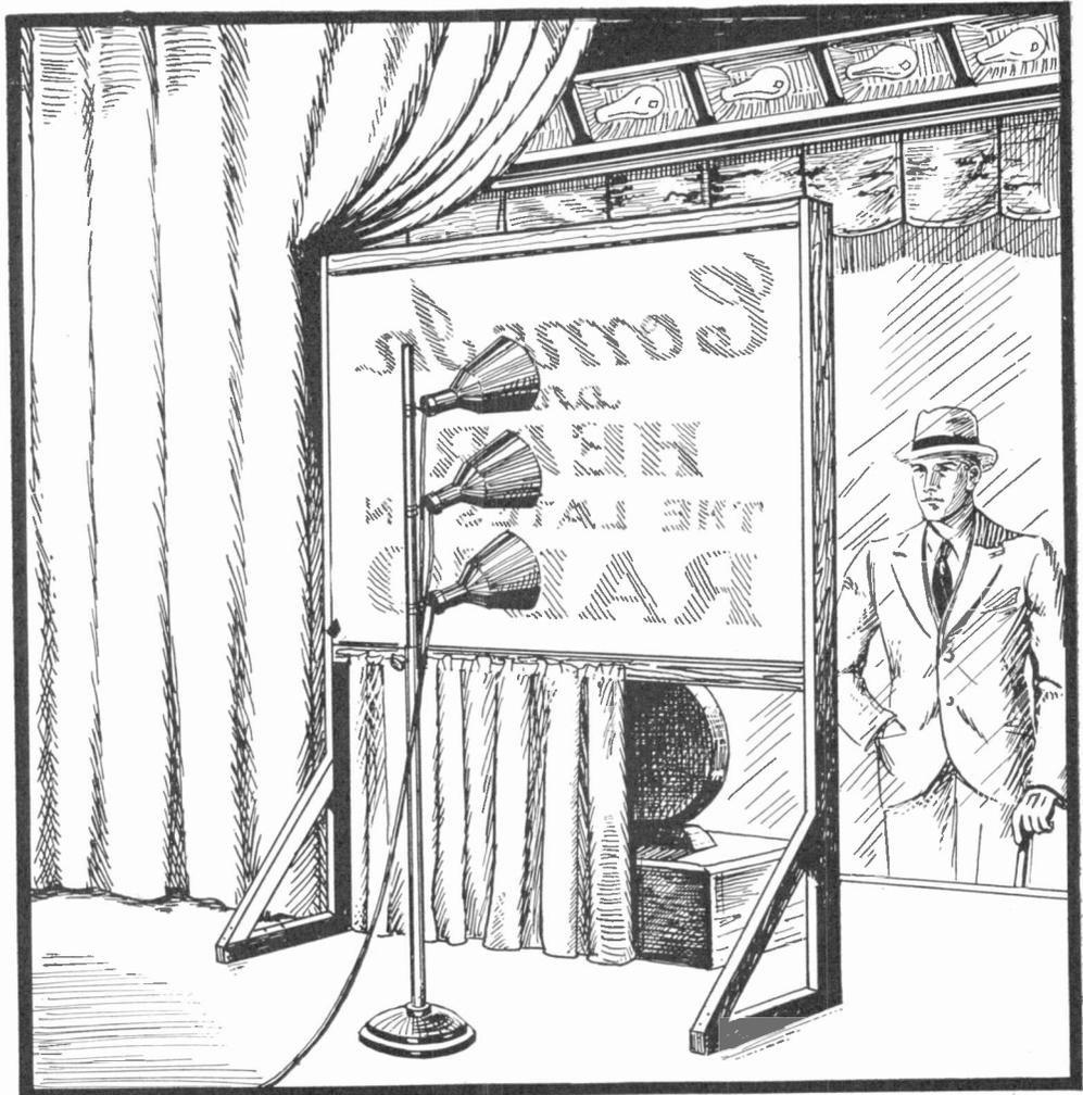
*This illustrates one way in which the contact panel board may be used. A spotlight plays on a muslin sign for a few seconds and is followed by a twinkling change of colors in the background. Many other different effects can also be obtained.*
