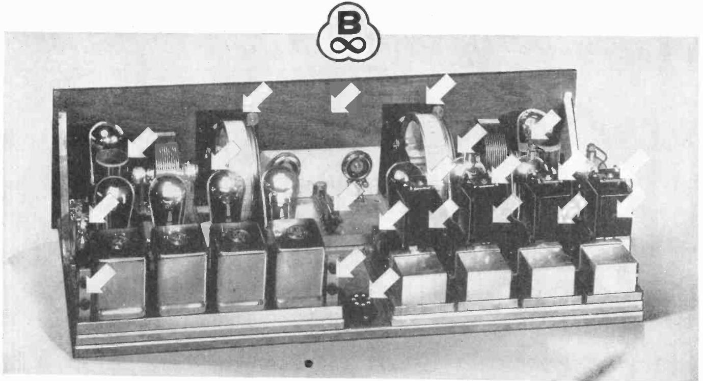
Isotone Receiver and Amplifier Chassis, showing some of the Bakelite Insulated parts. Made by High Frequencies Laboratories, Chicago.
