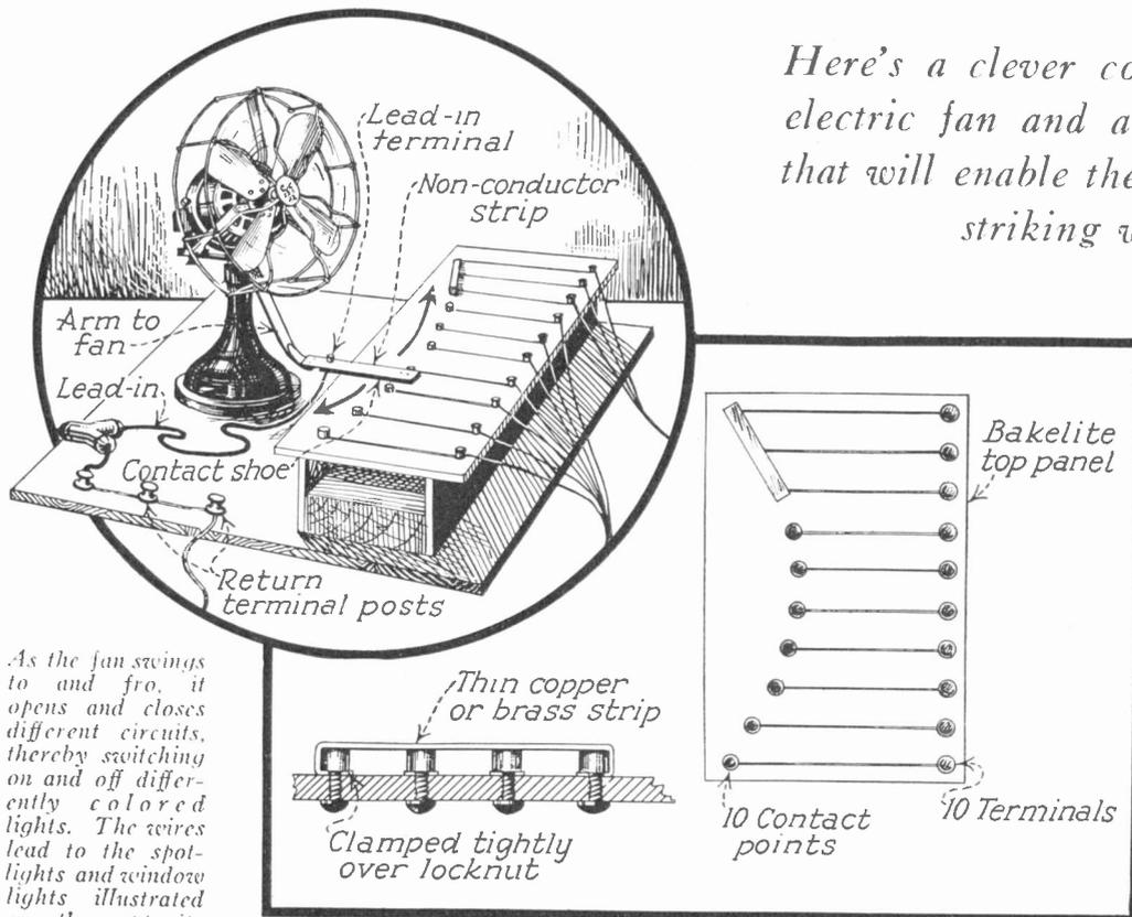
As the fan swings to and fro, it opens and closes different circuits, thereby switching on and off differently colored lights. The wires lead to the spot-lights and window lights illustrated on the opposite page.
