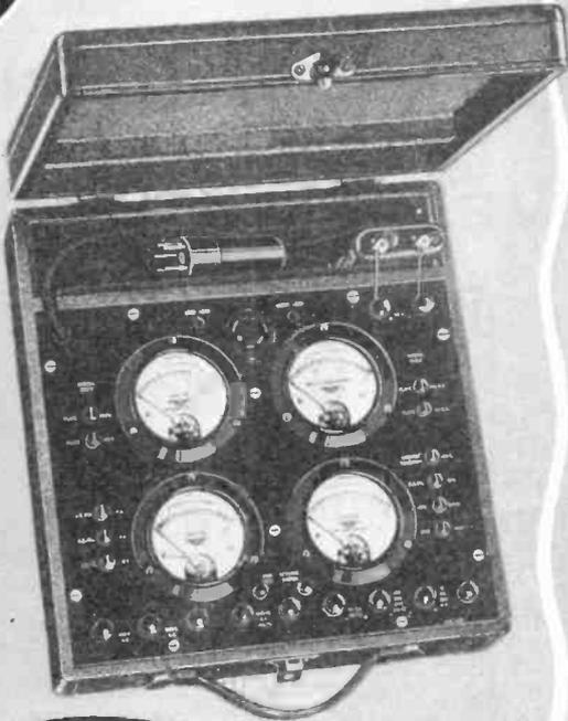
AGAIN Jewell takes the lead with a Set Analyzer that accurately meets service needs. In the Jewell Pattern 409 the dreams of expert radio servicemen are realized. This remarkable instrument gives filament, grid, and plate voltages, as well as plate current, simultaneously.
