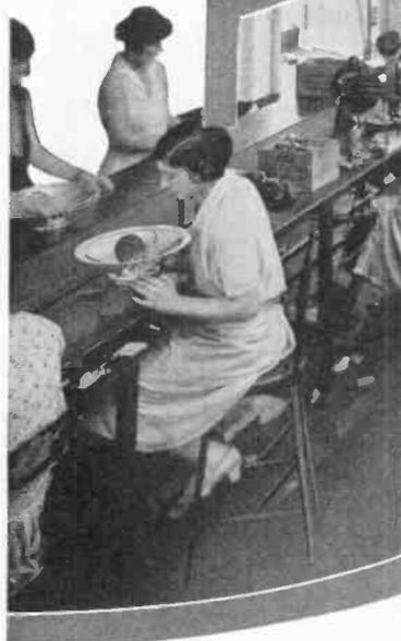
*Above:* The longest speaker assembly line in the world. Here precision parts made in the big Valley Plant are assembled into the complete chassis unit, tested, given final inspection. Thousands of chassis go over these lines every day.
