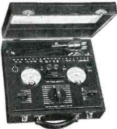
The Jewell Pattern 444 Set Analyzer allows rapid servicing of receivers employing even the most complex circuits.
