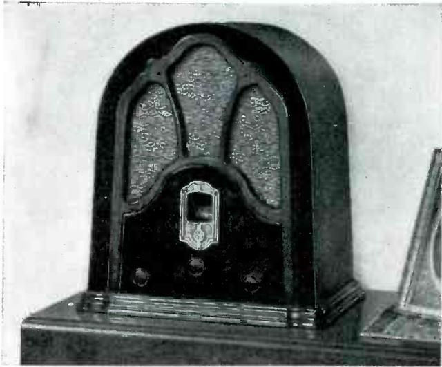
GENERAL ELECTRIC J-70 TABLE MODEL—A new cabinet style in full-size table models. An improved 7-tube superheterodyne with 2 super control tubes and Pentode output. Floating chassis—rubber mounted. Full range tone control. Dynamic speaker. New, distinctive two-tone cabinet with beautiful glossy finish. Instrument panel finished in dark burled walnut. Dimensions 17 1-4" high, 14 3-4" wide, 10 1-4" deep.
