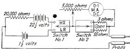
With switch No. 1 at HR and No. 2 in the open position (center) resistors and r.f. coils of from 10,000 to 1,000,000 ohms may be checked. 10,000 ohms will read 0.7 mils., r.f. coil primaries from 0.3 to 0.4 mils. For high voltage transformer windings set switch No. 1 at LR and leave No. 2 open. Readings should be from 0.7 to 0.8 mils. Half windings will show 0.3 to 0.4 mils.
