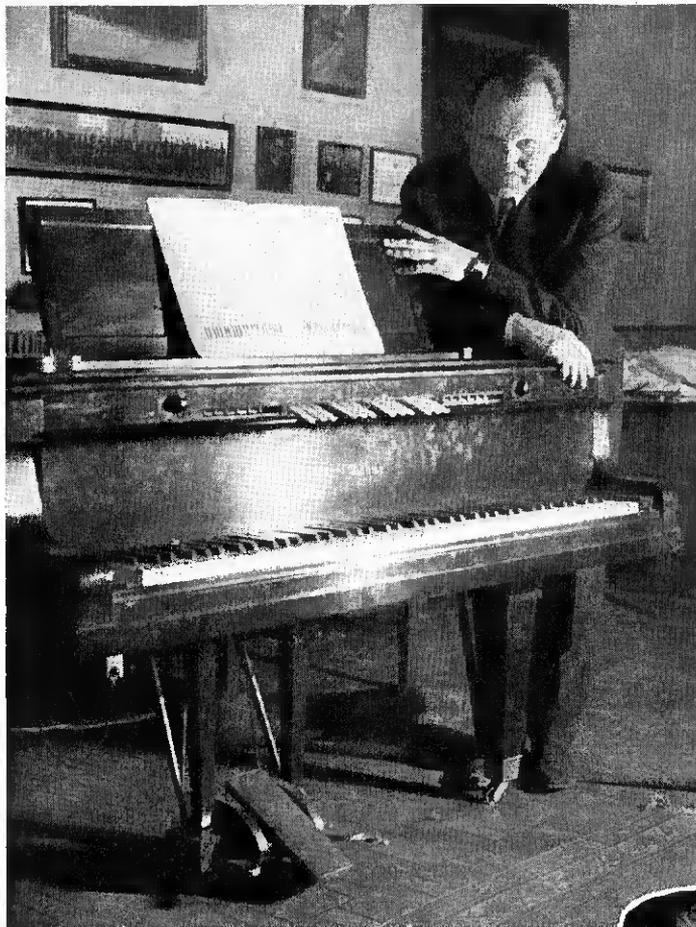
*This new Miessner instrument can be played as a piano and as an organ, and as the source of tones duplicating those of the flute, French horn, violin, piccolo, music box, etc. Piano strings are used as the source of the vibrations, which are then amplified and recombined electrically, and heard through a loud-speaker*
