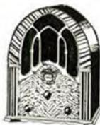
This 6-tube superheterodyne incorporates 2½-volt heater tubes—push-pull pentode output—double tuned image suppressor pre-selector—dynamic speaker and other outstanding features. Dimensions: 16¾" high, 13½" wide, 8½" deep. **\$38.50** Complete with tubes Plus Tax
