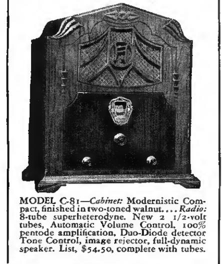
MODEL C-81—Cabinet: Modernistic Compact, finished in two-toned walnut. . . . Radio: 8-tube superheterodyne. New 2 1/2-volt tubes, Automatic Volume Control, 100% pentode amplification, Duo-Diode detector Tone Control, image rejector, full-dynamic speaker. List, \$54.50, complete with tubes.
