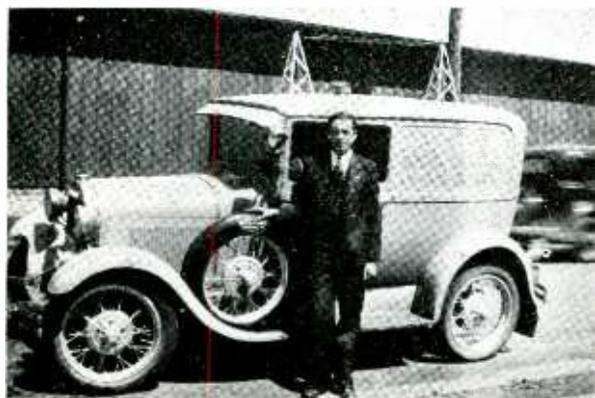
J. B. Jackson and the truck he uses when shooting interference. Note the miniature masts. This roof aerial attracts attention as well as supplying strong signals for an auto receiver
