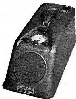
Model B-52 (Left)—G-E Portable Auto Radio. 5-tube superheterodyne that operates on car battery or 110-volt, 60-cycle A. C. Full, brilliant tone, particularly in higher registers. Low battery drain. Factory-sealed vibrator. High output and sensitivity. Airplane-type illuminated dial. Dimensions: 6½ in. high, 7½ in. wide, 17½ in. deep. Brown streamline case—crackle finish.
