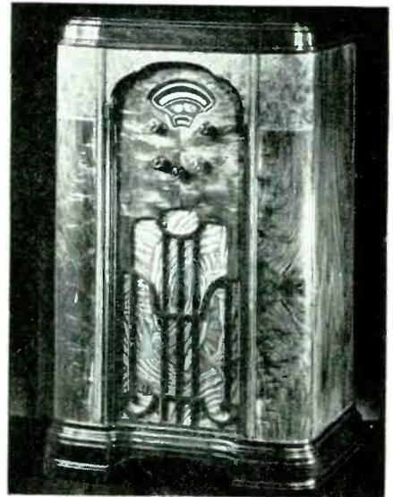
**ALL WAVE**—Model 559N—9-tube superheterodyne, 11 tuned circuits—range from 540 kilocycles to 18 megacycles in 4 bands, 6-section gang condenser, 2-speed tuning 6 to 1 and 60 to 1 ratios, 11-inch speaker, 4-position tone control has usual low medium and high tone pitches with *high* selectivity and 4th with *low* selectivity and high *faithful* tone reproduction. **\$135.00** f.o.b. factory.
