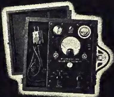
Model 669 - Vacuum Tube Voltmeter
