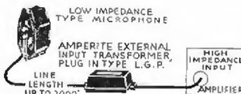
said to be entirely eliminated by the hum neutralization design of the transformer. Either a 50 or 200 ohm microphone may be fed into the standard input impedance of 200 ohms. Other impedances available upon request.—List price \$5.00—*Radio Retailing*, July, 1936.
