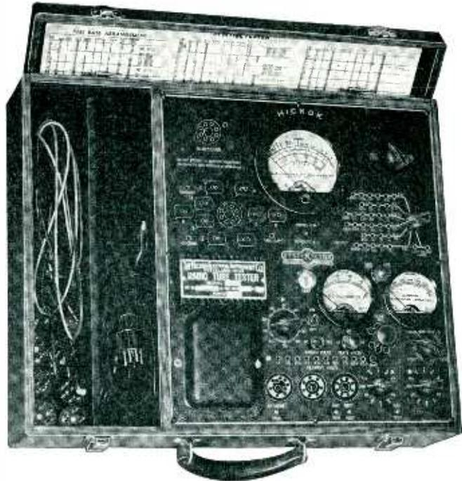
Combines both the static and dynamic method of set testing in compact and simple form.
