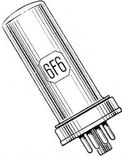
Normally the function of most tubes is to amplify a signal. But when tubes are required to deliver power, such as the 6F6, the amplification may test up and yet the tube may distort badly. Reason . . . weak emission . . . particularly at low frequencies. Such tubes demand both amplification and emission test, now available
