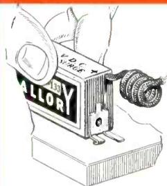
Half of flange may be bent down to fit in any convenient chassis hole.
