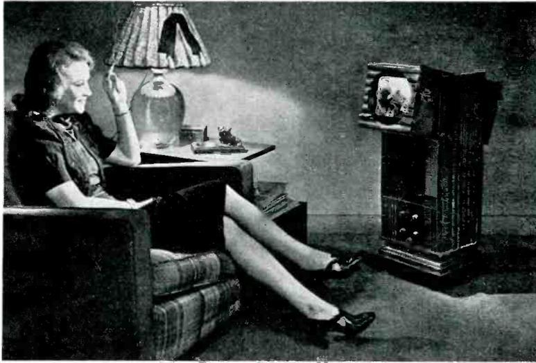
**EXTENSION TELEVISOR**—What an extension speaker is to radio American Television Corporation's "kinet" may be to television. Portable, adjustable, equipped with its own cathode-ray tube and magnifying lens, the pictured accessory works from the output of a television receiver elsewhere in the home
