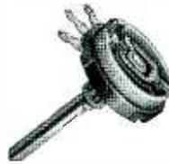
**CONTROLS**—Low power wire wound controls and rheostats are made in all needed ranges up to 10,000 ohms. They are equipped with "Silent Spiral Connector" which provides positive, continuous contact between rotor arm and end terminal. Power dissipation is 2 watts. Units are available with or without switch, and with complete assortment of shaft variations for any manufacturing or service replacement requirement. Diameter 1/4 in. by 1/8 in. depth of case.
