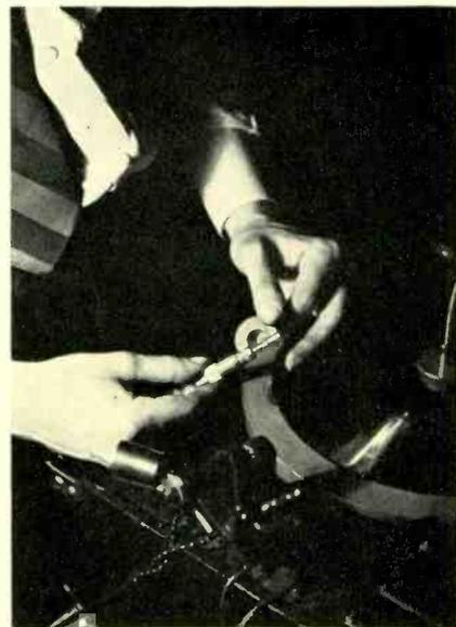
**MEASURE THREAD THICKNESS**—One way to be sure cuts are correct is to measure the diameter of the resulting “thread” with a micrometer. Standard for most acetate materials is .015 in.
