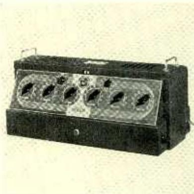
**AMPLIFIER**—Uses beam power tubes, four channel input, electronically mixes three microphones simultaneously with phono input, provision for Remote Controller, volume expansion, volume compression, electronic visual overload and output level, indicators nonresonant equalizer used as tone balancer for high and low frequencies, master gain control, six stages, thirteen tubes, 55 watts output at 5 per cent distortion. *Radio and Television Retailing, June, 1939.*
