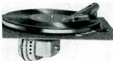
PHONO MOTORS—Model KX, CX and RX, self-starting, induction type motors. Model KX and CX are fully enclosed, ventilated and fan cooled, have silent helical-cut gears, gears and bearings run in oil. Patented combination metal and rubber drive. Model KX3 is geared for 33 1/3 r.p.m. as is model CX3. Model RX is rim-drive, insulated from mounting plate, as is CX and KX. *Radio and Television Retailing, June, 1939.*
