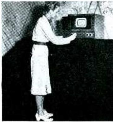
**TELEVISION RECEIVER** — Incorporating the new flat face picture tube with the "ion trap" which eradicates the dark spot found in the center of the television picture. Also transmits television sound to standard broadcast radios. *Radio and Television Retailing, July, 1939.*
