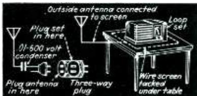
from one side to ground. When such sets are used in the vicinity of line antenna sets this condenser will bypass nearly all r.f. in the line.
