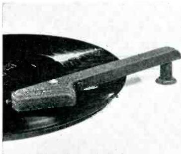
**CRYSTAL PICKUP**—Model X-79A phono pickup with convenient single mounting hole fastener; may be used on motorboards 1/16 to 1/2 inch thick. Frequency response stated to be 50 to 8500 cycles; 2.5 ounce needle pressure. Arm assembly is rubber cushioned eliminating microphonic feedback and motor noises. Available with or without built-in pilot light. Webster Electric Co., Racine, Wisconsin.
