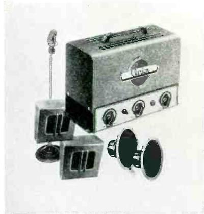
**SOUND SYSTEM**—Medium powered complete sound system, model C-418. Rated at 16 watts; 113 db. gain on mike input; 60 db. gain on two phono inputs; response 40 to 9500 cycles; output tapped from 2 to 500 ohms. With two 10 inch p.m. speakers in wall baffles, mike, floor stand, all cables and plugs, \$99.98 list. Transformer Corp. of America, 69 Wooster St., New York, N. Y.
