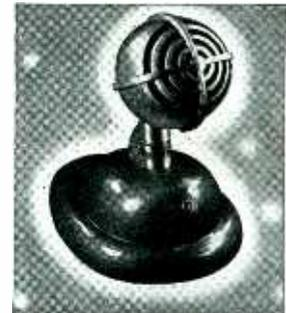
**SHURE** MICROPHONE, "Uniplux" Cardioid crystal cuts down room noise pick-up. Model 7305 has built-in r.f. filter which protects against burnouts. Output level—33 db. below 1 volt for 10 bar speech signal. Swivel head. Satin chrome finish. Diameter 3 1/8 inch. Depth 3 3/8 inch. Complete with 7 ft. super-shielded cable. Available in Model 7305H at \$32.50 list; also in Model 7305, complete with desk mount, at \$35.50 list. Shure Bros., Microphone Headquarters, 225 W. Huron St., Chicago, Ill.
