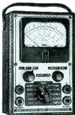
**PRECISION** MULTI-RANGE TESTER, series 834, equivalent in size to a man's hand, offers 18 voltage ranges, 0-12/60/300/600/1200/6000 in ac-dc and power output, at 1,000 ohms per volt; 4 current ranges, 0-1.2/12/60/600 mls; 3 resistance ranges, 0-5M/500M/5 megs; and 6 decibel ranges from -10 to +70 db. Precision Apparatus Company, 647 Kent Ave., Brooklyn, N. Y.
