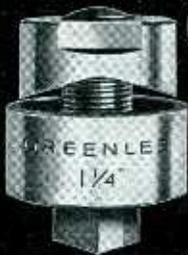
Here's a handy tool to help the radio worker save many hours of work when cutting holes for sockets, plugs, connectors, and meter holes in radio chassis. No tedious drilling, reaming, or filing is necessary. A cap screw is inserted in a small drilled hole, and the punch is easily forced into the die by a few turns of the cap screw with an ordinary wrench. Ten punches are available for cutting 3/4, 7/8, 1, 1 1/8, 1 1/2, 1 3/8, 1 1/4, 1 3/8, 1 1/2 and 2 1/4-inch holes. Write for more information.
