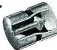
Note in cutaway, baffle at end of electrode. Prevents splashing of mercury. Keeps light flicker-free. Central position of electrode makes it instantly operative in any position. For low-voltage circuits up to 25AC or DC, up to 10 amps. at 6 volts, and 5 amps. at 25 volts. For lights, in auto glove compartments, trunk, hood—radio, refrigerator door lights, pin games—many and varied services.
