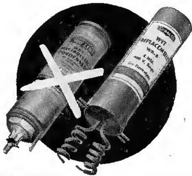
**SPRAGUE TYPE WR** tubular cardboard dry electrolytics replace wet capacitors and also various aluminum can dry types. Have high voltage formation to insure their standing up under the high peak voltages impressed on wet electrolytics. Diameter is same as standard wets. Available in 3 sizes—WR-8 to replace capacities from 4 to 8 mfds., WR-16, capacities from 12 to 18 mfds. and WR-25 from 20 to 40 mfds. Sprague Prods. Co., North Adams, Mass.—RRT.
