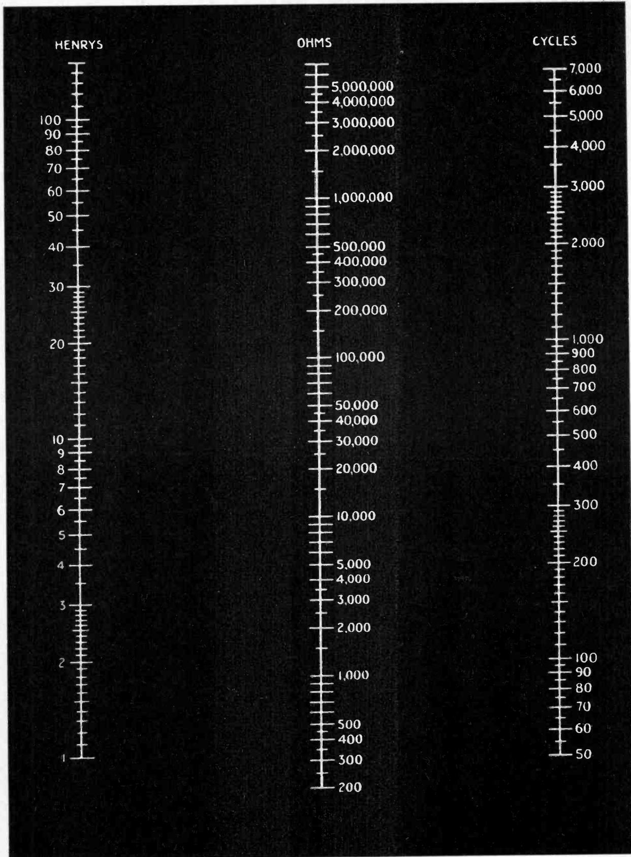
Knowing any two of the factors, inductance, ohms reactance, or frequency, you can determine the third by placing a straight-edge between the points of known value; the intersection with the third scale gives the unknown. To expand the scales, multiply the frequency scale by any number and divide the inductance scale by the same number. Ohms scale is unchanged.
