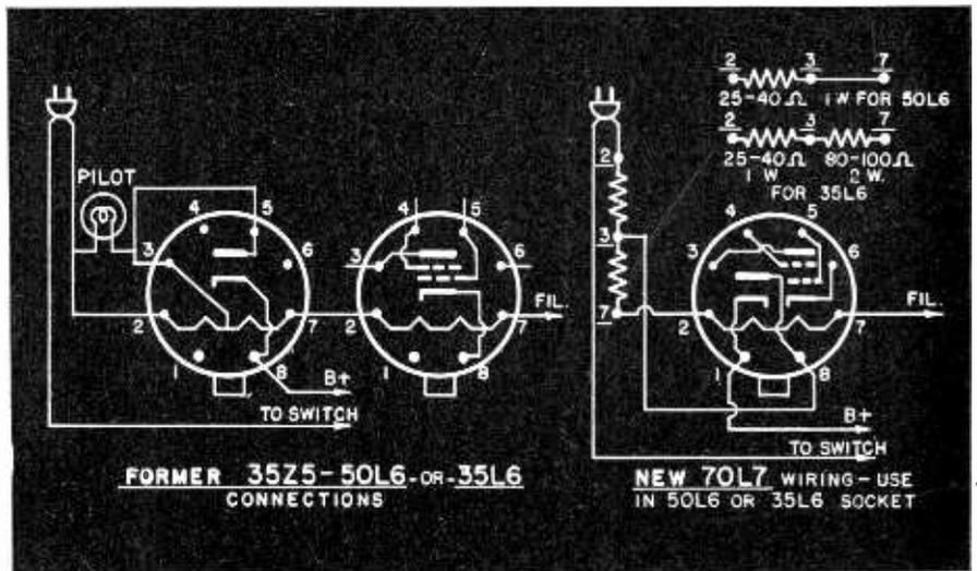
Fig. 3—The popular 35Z5-50L6 combination of rectifier and output tube can be successfully replaced with a 70L7 used in the 50L6 or 35L6 socket which will save considerable rewiring. If a 50L6 was used, connect a 25-40 ohm resistor between the pins 2 and 3 on the unused 35Z5 socket and connect a jumper between pins 3 and 7. If a 35L6 was used, put a 25-40 ohm resistor between lugs 2 and 3 and 80 to 100 ohms between 3 and 7.
