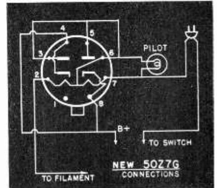
Fig. 2—The 50Z7G can be used to replace a 35Z5 if the connections are made as shown here.
