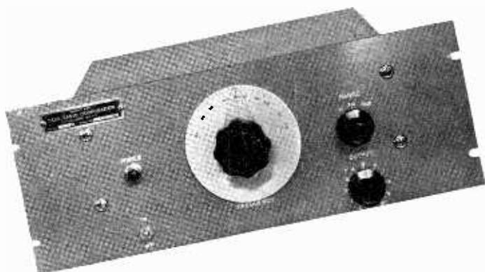
A precision sine wave audio oscillator which at the flip of a switch gives square wave output . . . radically new . . . product of Fada war-time engineering research . . . just one of an extraordinary variety of different equipments today produced directly for many services of our government in FADA'S modern, fully mechanized radio/electronics plant.
