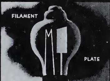
9 Electrons flow best in a vacuum, Dr. Irving Langmuir of General Electric found in 1913. In its simplest form, the airtight tube has two elements: filament and plate.
