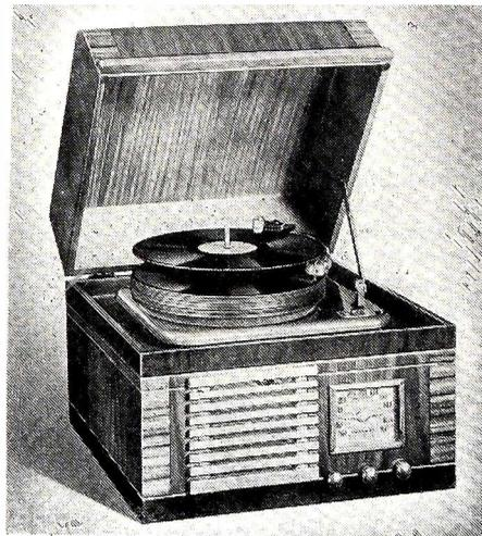
Model C-107 is a 6-tube (including rectifier) ac superhet radio-phonograph console. Has 8" electro dynamic speaker. 3-dimensional dial. 3-gang condenser; tuned r-f stage for greater efficiency. Features are pull-out phonograph drawer, record album compartment. Automatic record changer with jam-
