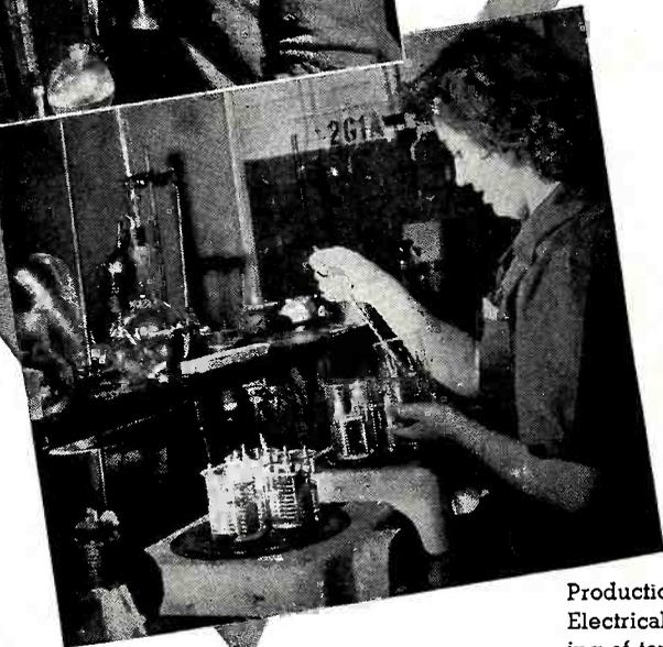
Production control of impregnating materials. Electrical test is preceded by careful checking of temperature of oils.
