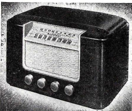
Model 294-T is a 6-tube ac-dc superhet. Receives on two bands. Has 6" permanent-magnet dynamic speaker; automatic volume control. Among features are built-in loop antenna, full range tone control, slide rule dial. Beam power output. Cabinet is of walnut veneer. Shipping weight is about 11 pounds. Measures 15" x 9<sup>3</sup>/<sub>8</sub>" x 7<sup>1</sup>/<sub>8</sub>". Sentinel Radio Corp., 2020 Ridge Ave., Evanston, Ill.—RADIO & Television RETAILING
