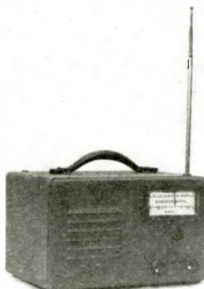
ready 762 or equivalent and 8 regular flashlight batteries. Removable corrosion-proof telescopic antenna, (10" to 40") PM dynamic speaker. Full vision slide rule dial. Drip-proof construction, leather handle, all metal cabinet cadmium plated. Navy gray crackle finish with blue escutcheon and knobs. Measures 11 1/2" long, 7" high, 8 1/4" deep. Soundview Radio & Television Corp., 86 Hugh St., Bronx, N. Y.—RADIO & Television RETAILING
