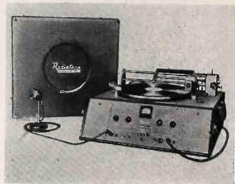
dynamically balanced. Drive shaft of hardened steel revolving on single steel ball. Instantaneous locking lever, speed shift from 78 to 33  $\frac{1}{3}$  RPM; directional of cut optional at will—lines per inch variable from 90 to 130 with calibrated indicator. Amplifier has phase inversion, inverse feedback and tone equalization; 12" PM speaker. Ellinwood Industries, 150 W. Slauson Ave., Los Angeles 3, Calif.—RADIO & Television RETAILING
