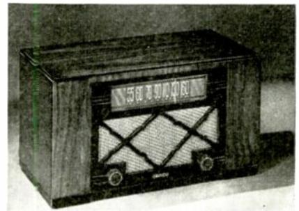
matic volume control, large slide-rule dial for glider tuning. Battery pack (1,000 hour) enclosed in cabinet. Walnut cabinet with stained trimmings and grille. Garod Radio Corp., 70 Washington St., Brooklyn 1, N. Y.—RADIO & Television RETAILING
