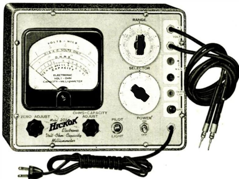
This new Hickok Model 203 is much more than an improved volt-ohm-milliammeter for it also measures capacity and inductance.
