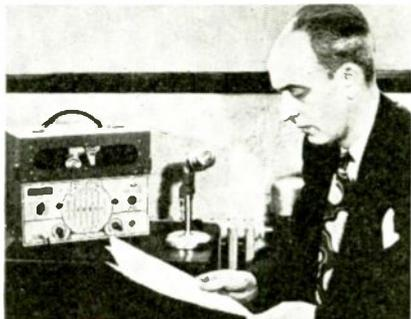
via converter). Wire lasts indefinitely; "erasure" of previous recording is automatic. Can be used as PA system—with high impedance microphone or phono turntable and auxiliary speaker. Welded steel case construction, silver grey wrinkle lacquer finish, rubber feet, carrying handle. \$595, including desk-stand microphone (plus \$40.16 Federal tax). Bell & Howell Co., 7100 McCormick Rd., Chicago 45, Ill.—RADIO & Television RETAILING
