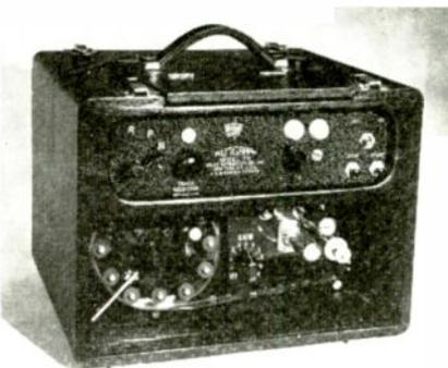
40 ft. Three-position control for recording, play-back and public address. Both speed and volume control for play-back. Permanent type sapphire stylus in dual purpose head for both recording and play-back. Manufacturer states Filmgraph is designed for authorized telephone recording. Luggage type cabinet, 11½" deep, 9½" high, 13" wide. Weighs
